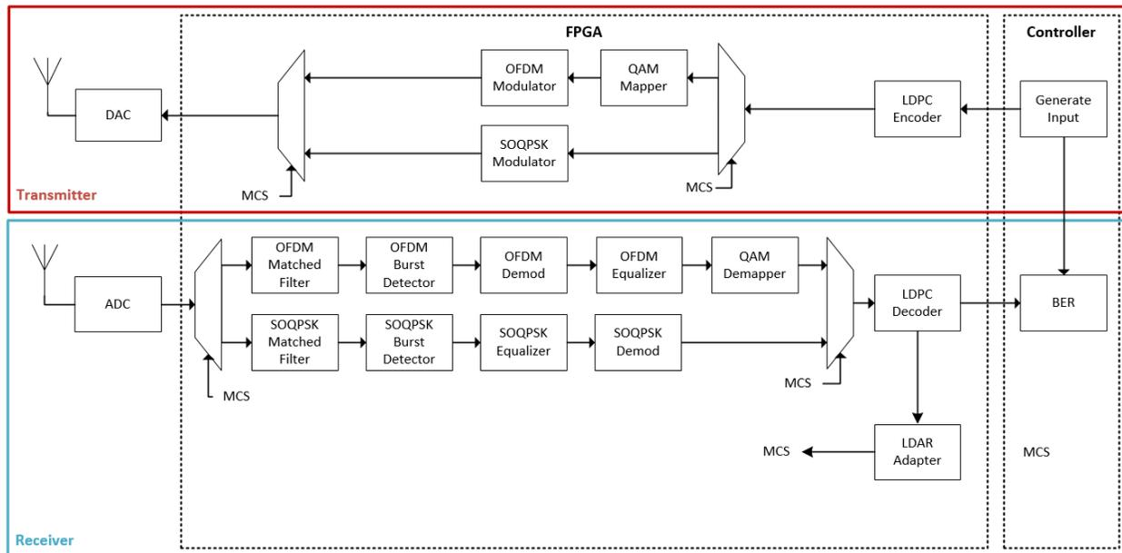
**Figure 8: Top-level architecture for next generation LDAR transceiver.**
