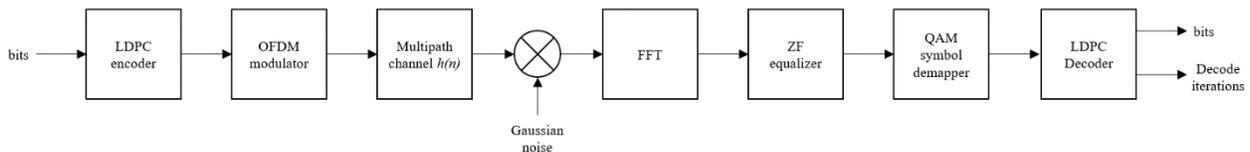
**Figure 4. Block diagram for OFDM simulation.**
