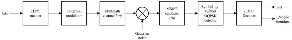
**Figure 3. Block diagram for the simulation procedure.**
