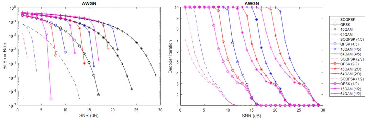
**Figure 2. BER and decoder iteration counts for all LDAR MCS selections.**
