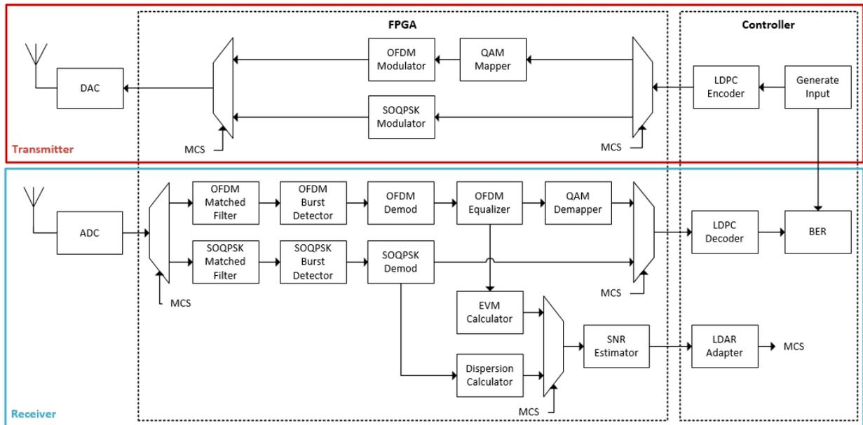
**Figure 1. LDAR transceiver top-level system diagram.**
