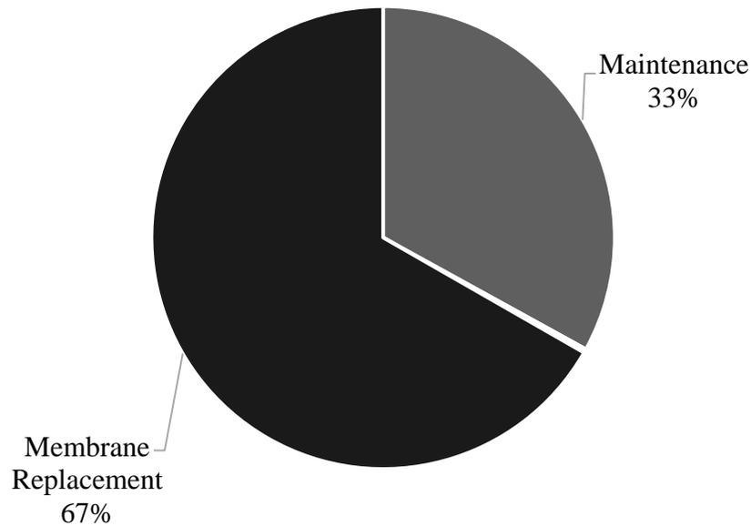
**Figure 5. Average annual operating cost breakdown for the optimized SMD system. The operating cost averages \$1,700 per year. Maintenance expenses include costs associated with routine replacement of fittings and minor equipment. The cost of labor for maintenance and brine disposal was also included in this calculation, but made up a negligible fraction of the operating expenses.**
