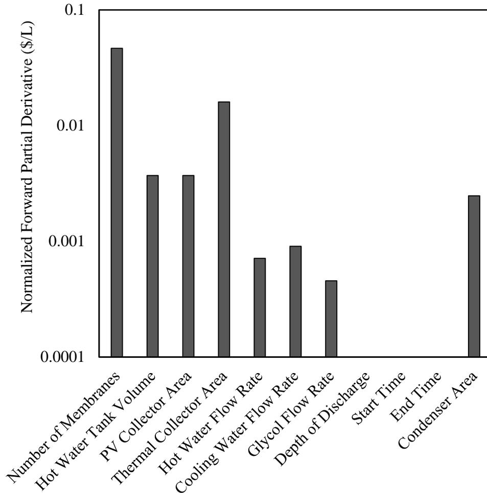
Figure 11. Normalized forward partial derivatives of the amortized cost of water near the optimum with respect to each decision variable.
