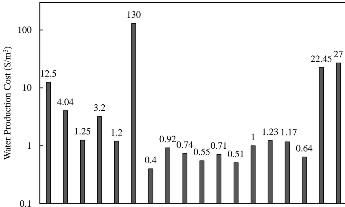
**Figure 1. Reported membrane distillation water production costs. System configuration, energy source, and methods for cost calculation varied. Details are given in Khayet (2013). In this data set, water production varied from 0.017 m³/day (\$130/m³) to 24,000 m³/day (\$1.17/m³).**
