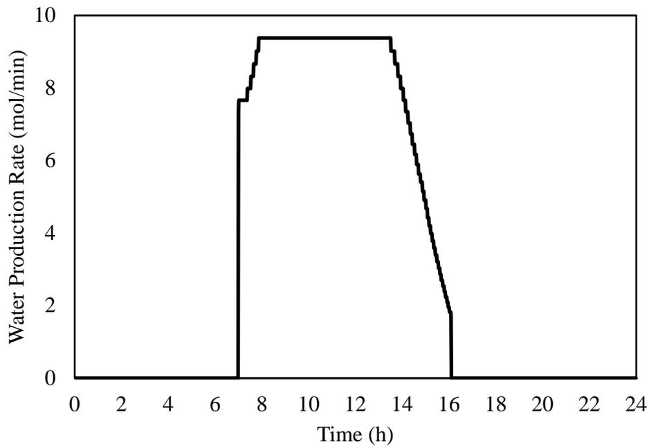
Figure 9 (top). Hot water tank temperature as a function of time for one day of operation in the optimal SMD system. Figure 9 (bottom). Water production rate as a function of time for one day of operation in the optimal SMD system. Time = 0 hours represents 12 am, while T = 24 hours represents 12 am of the following day.
