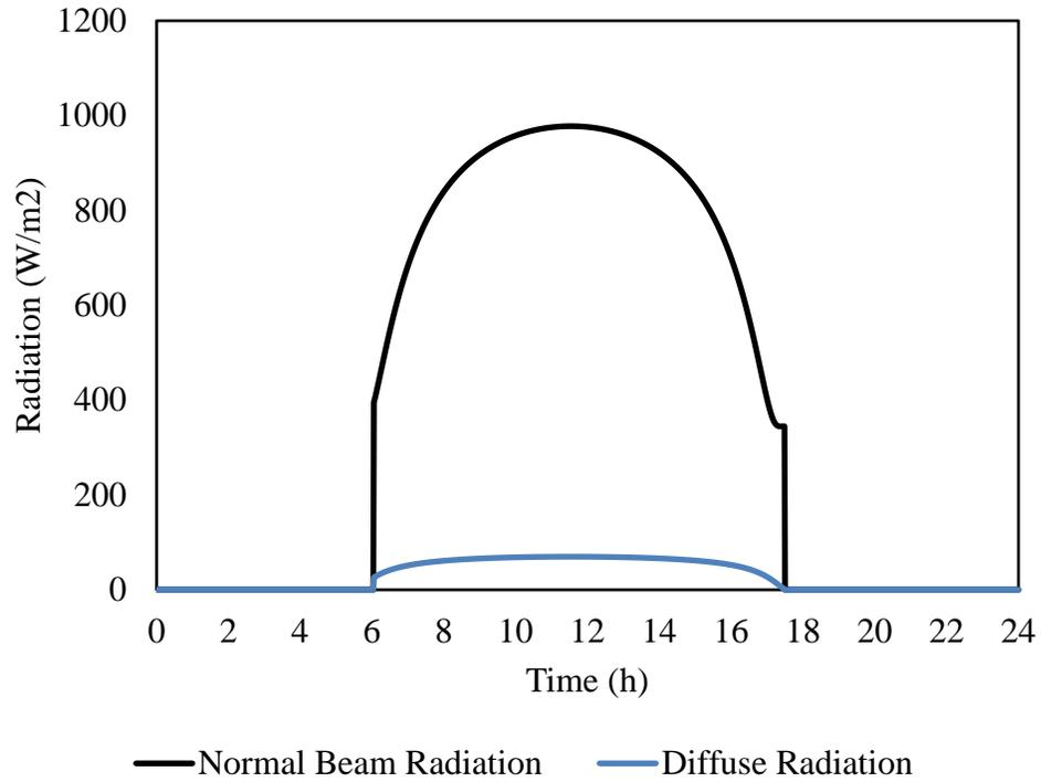
**Figure 6.** Clear sky ground level solar irradiation as a function of time for one day of operation (March 20 in Leupp, AZ). Time = 0 hours represents 12 am, while T = 24 hours represents 12 am of the following day.
