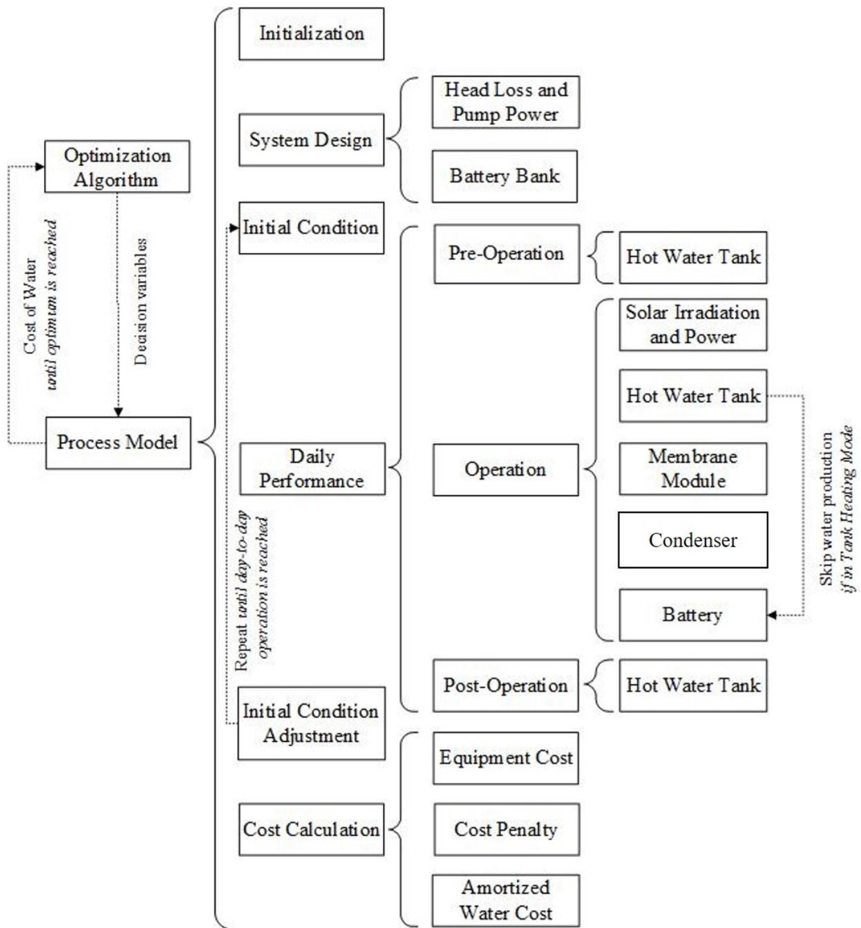
Figure 2. Optimization and process model schematic.
