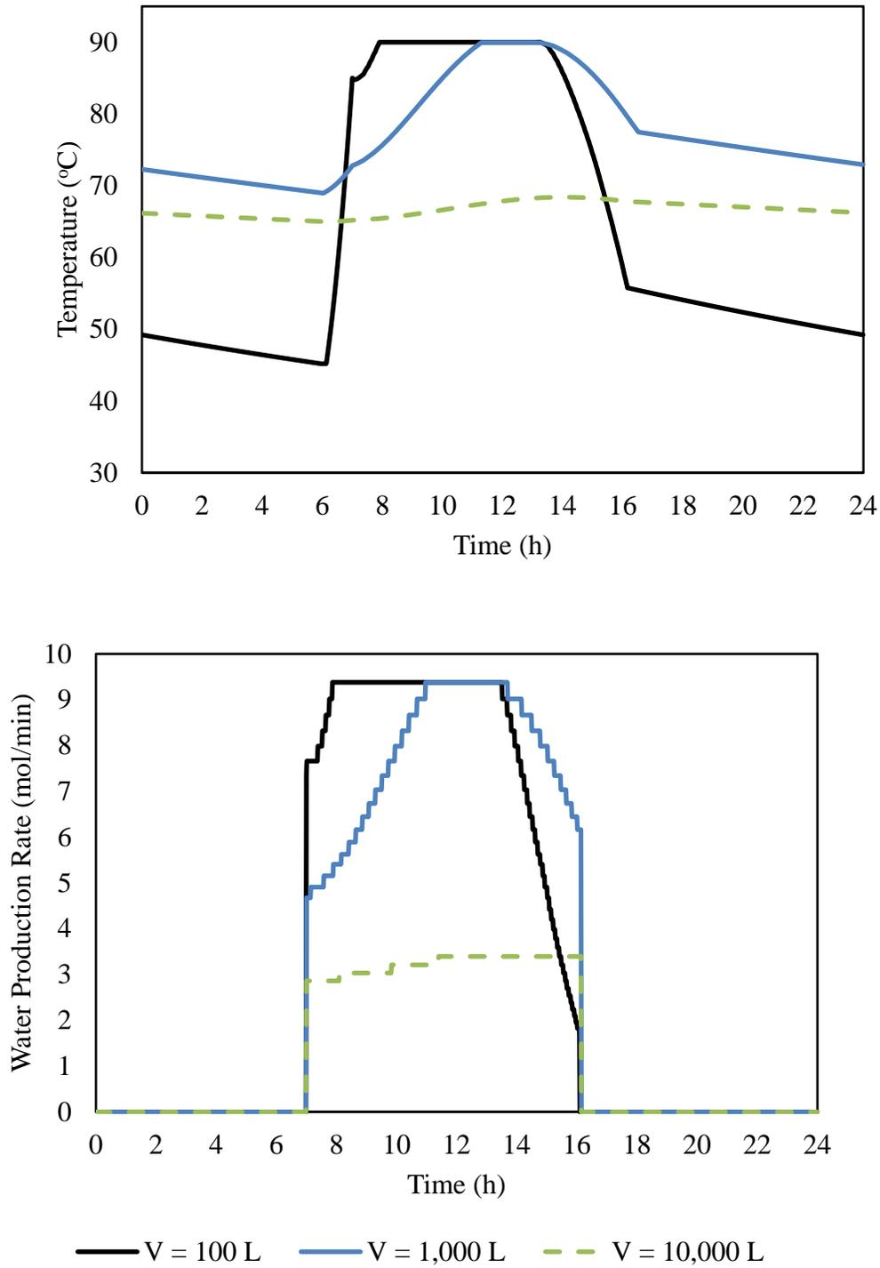
Figure 10 (top). Hot water tank temperature as a function of time for one day of operation using three different hot water tank sizes.
