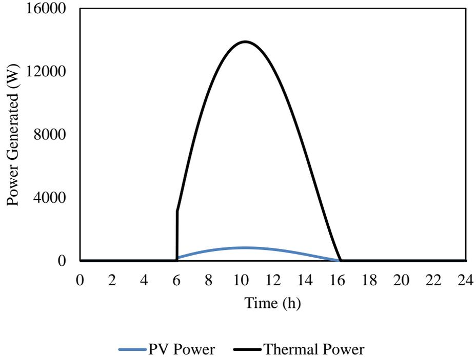
**Figure 7.** Thermal and electrical power generated as a function of time during one day of operation (March 20 in Leupp, AZ). Time = 0 hours represents 12 am, while T = 24 hours represents 12 am of the following day.
