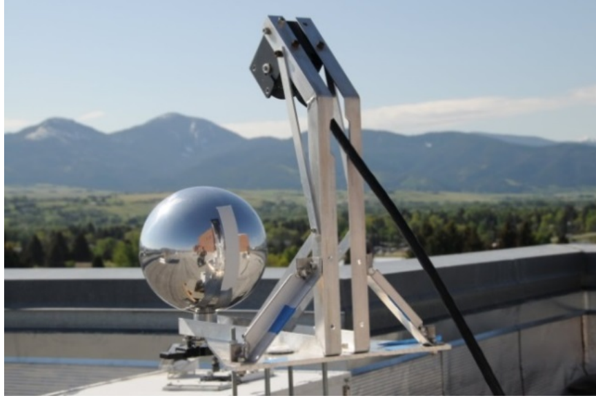
Fig. 1. The reflective all-sky ICI uses an aluminum sphere to reflect the whole sky into a low-cost LWIR camera in an off-axis position to avoid blocking the zenith sky.
