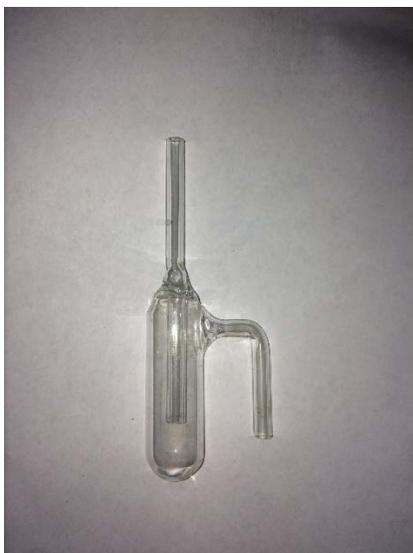
Figure 2.3.1. Specialized glass sample cell used for the microwave experiments in this dissertation.
