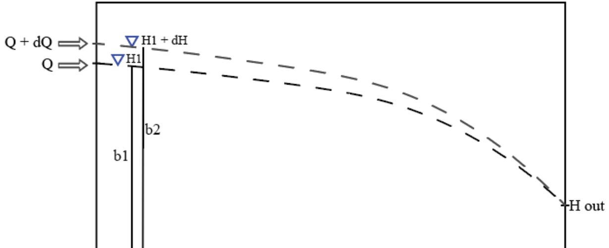
**Figure 9.** The unconfined aquifer system responds to a change in the flow in by changing both the head gradient and the saturated thickness.
