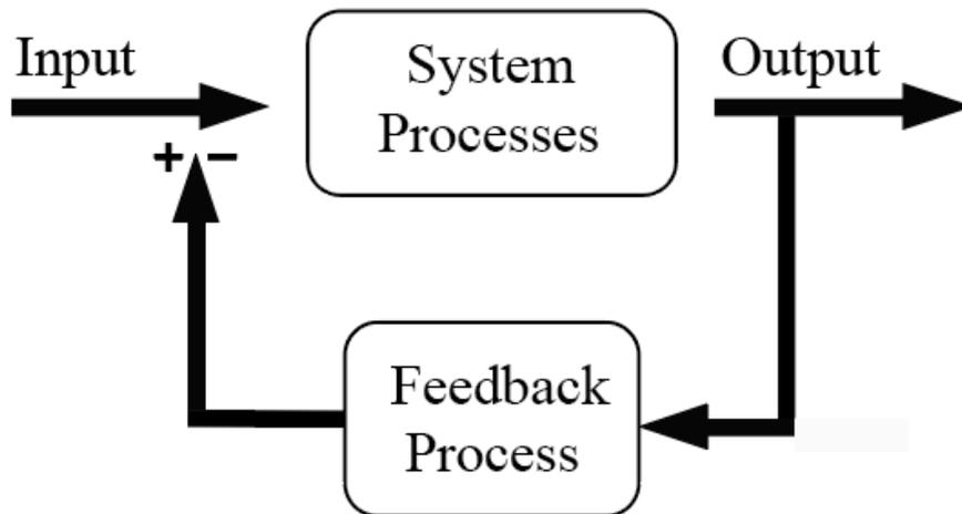
**Figure 2.** A more complicated system with an information loop that takes a signal from the output and then influences the input.
