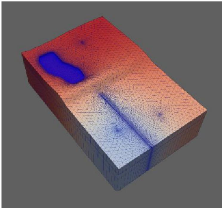
**Figure 10.** Illustrative model grid with ET flux shown as color flood.
