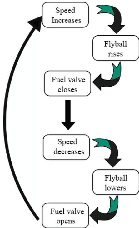
**Figure 5.** This conceptualization of the centrifugal governor’s process of maintaining a constant target speed shows two possible loops that are connected in an endless back and forth to establish a stable, constant speed through a negative feedback.
