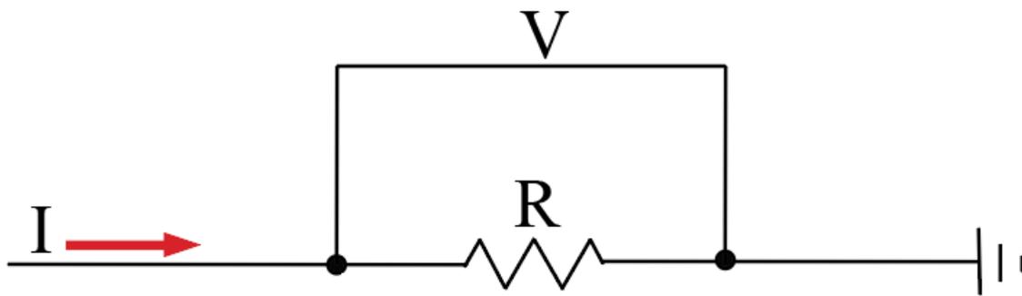
**Figure 7.** A simple electrical circuit with voltage shown across a distance with resistance  $R$  and current  $I$ .
