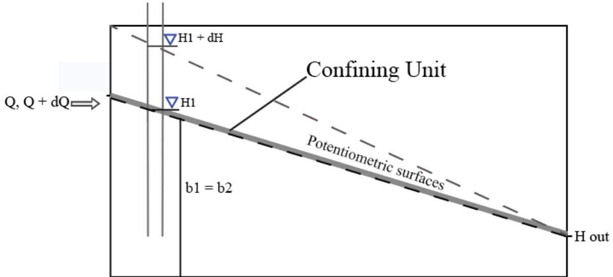
**Figure 8.** The confined aquifer system responds to changes in the amount of flow into the system by a change in the potentiometric head gradient, but the saturated thickness is constant.
