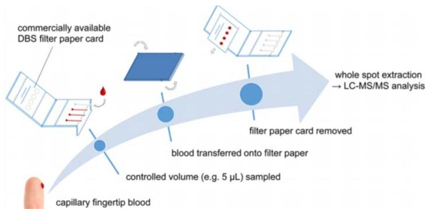
**Figure 20.** The new microfluidic-based sampling procedure offering DBS card on one side of the foldable structure and sized capillaries allowing a specific amount of whole blood to be absorbed on the other. The blood is supplied to the capillary side, a controlled and set amount of volume is absorbed, the device is closed and the blood is added to the DBS card. The whole blood spot is punched out and used for analysis [71].
