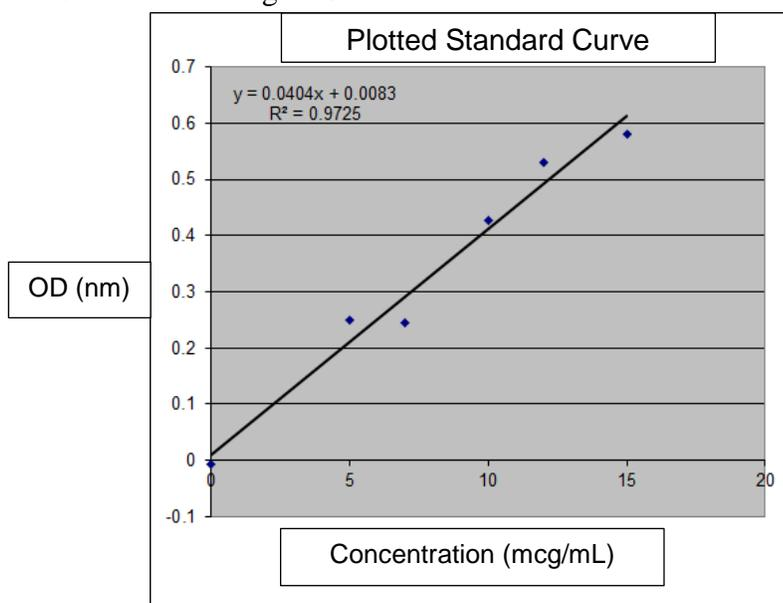
**Figure 5c.** Example of a plotted standard curve. The equation is used to determine the amount of lysate to use in the ELISA assay (to normalize protein concentration between samples).
