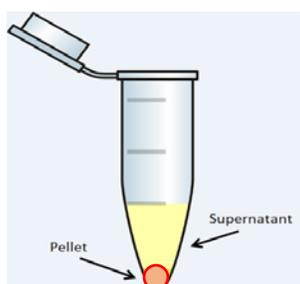
**Figure 5b.** Example of pellet and supernatant in a polypropylene microcentrifuge tubes (actual procedural aspiration occurs with supernatant and pellet in a conical tube) [18].
