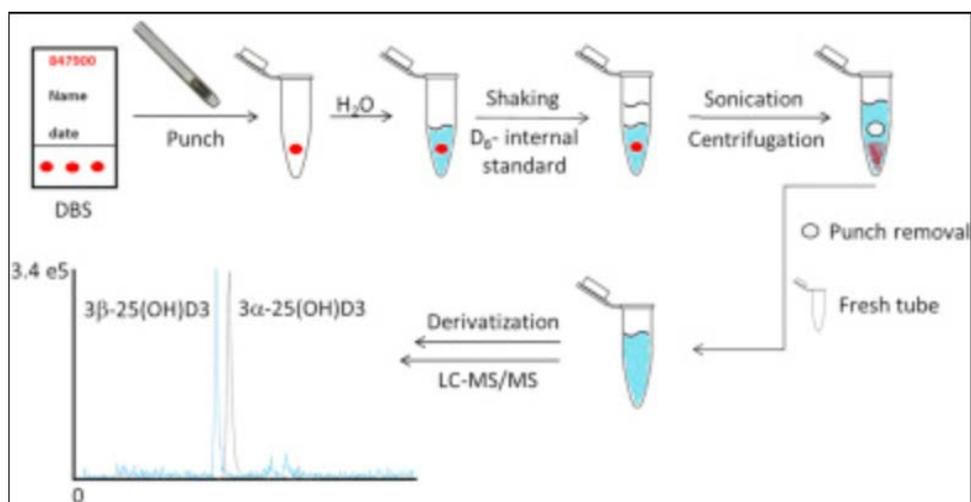
**Figure 12.** A generalized procedure for extracting dried blood spot punches for use in liquid chromatography mass spectrometry (LC/MS) [48].
