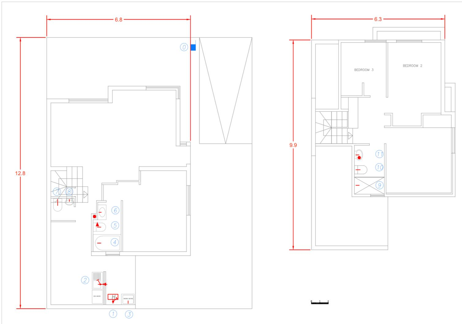
Figure 12: house 1 plan, including the nodes for each fixture in the cold system. Measurement in meters
