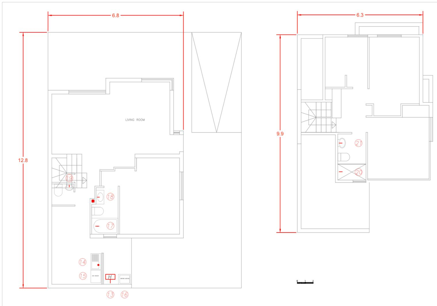
Figure 13: house 1 plan, including the nodes for each fixture in the hot system. Measurement in meters
