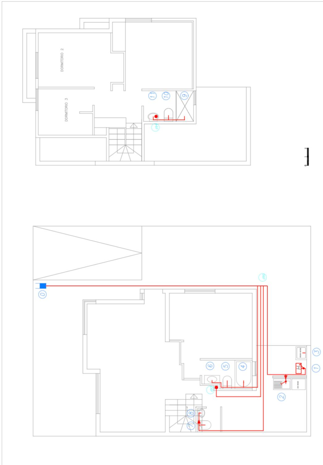
Figure A-9: house 1, layout 5 for the cold system
