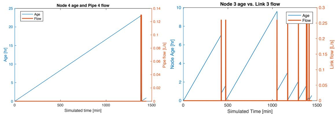
Figure 10: Age results for nodes 4 and 3 when increasing pipe lengths
