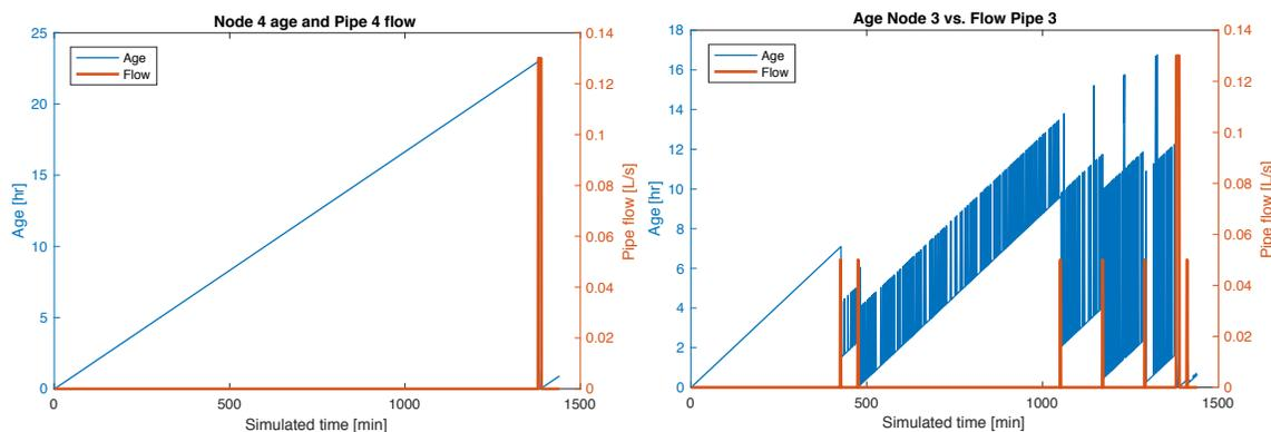
Figure 5: Resulting ages when closing pipes connecting to dead ends
