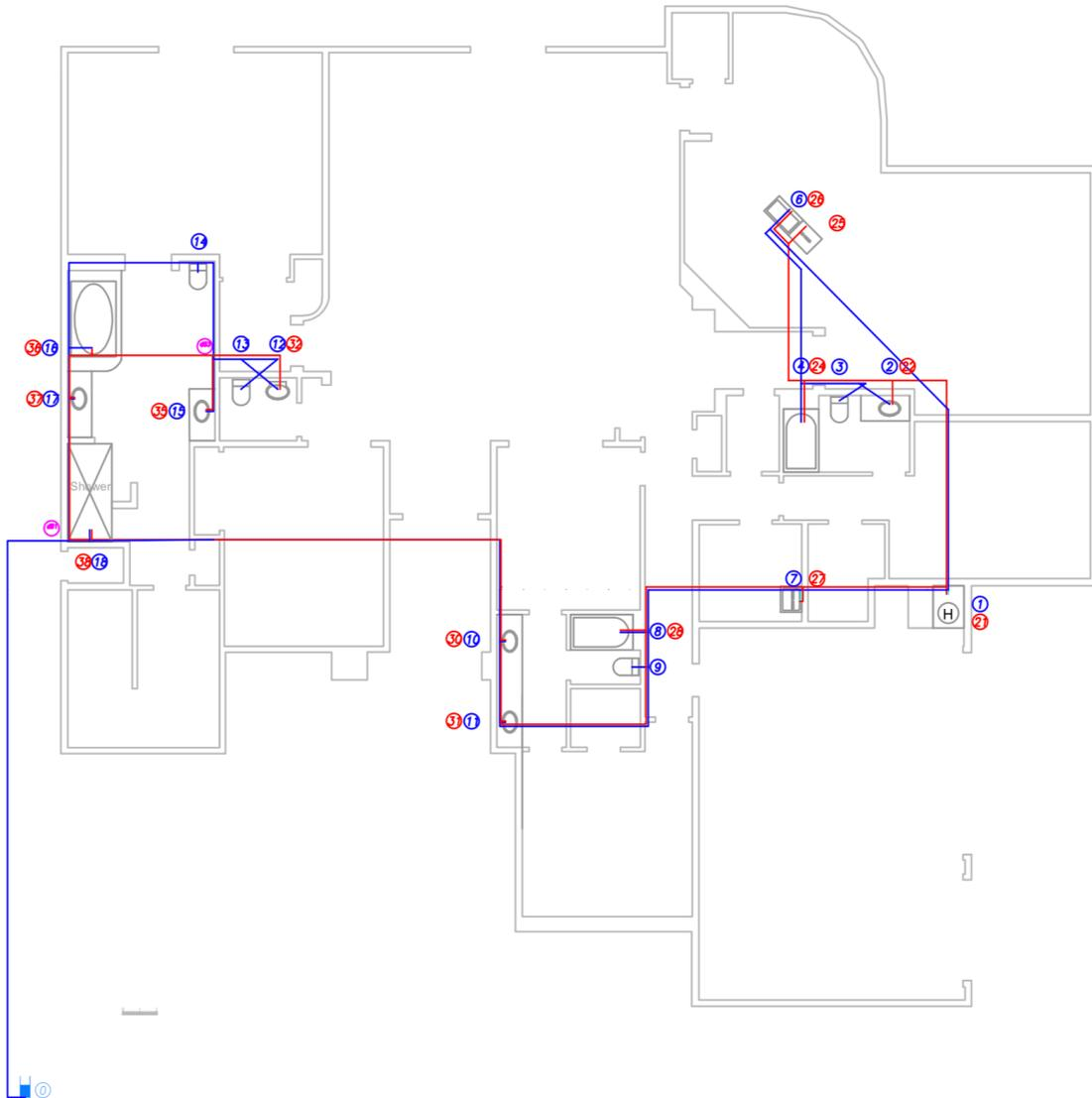
Figure A-13: house 2, layout 3 for both hot (red) and cold (blue) systems
