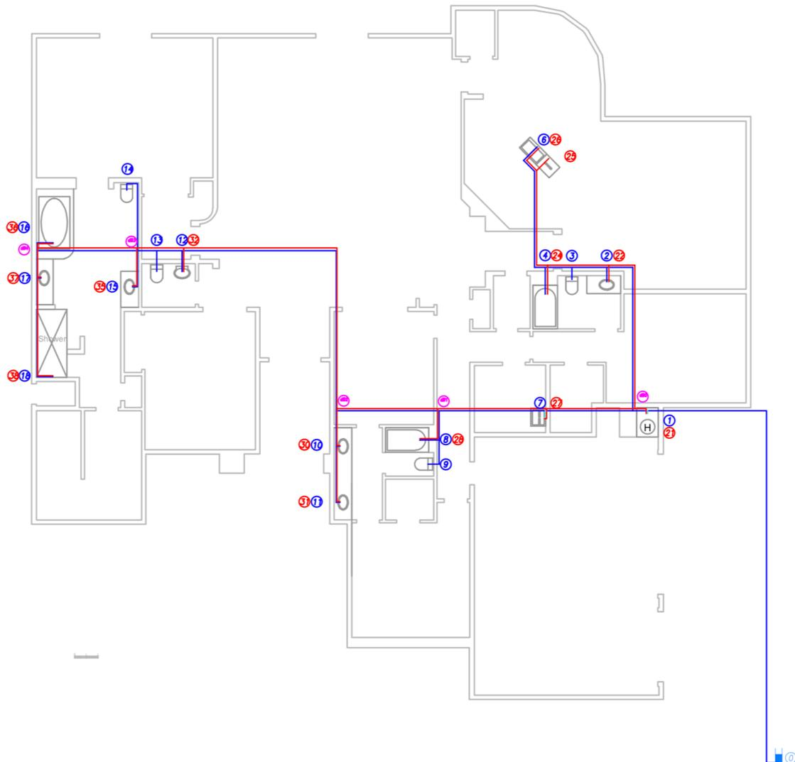
Figure A-11: house 2, layout 1 for both hot (red) and cold (blue) systems
