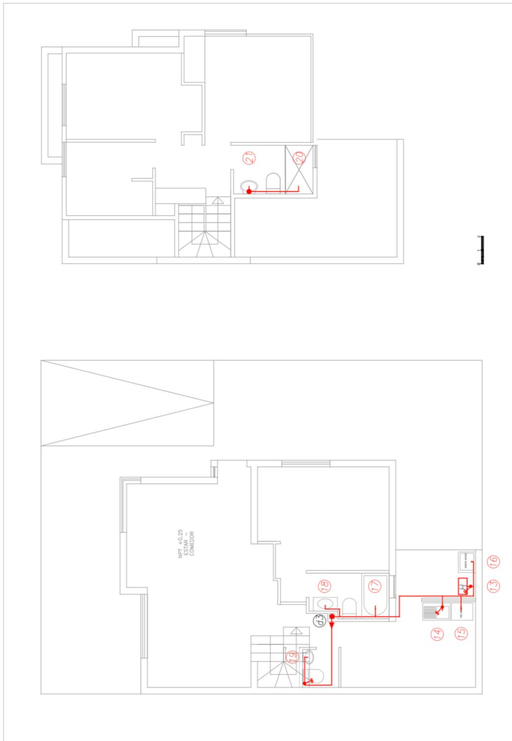
Figure A-2: house 1, layout 1 for the hot system
