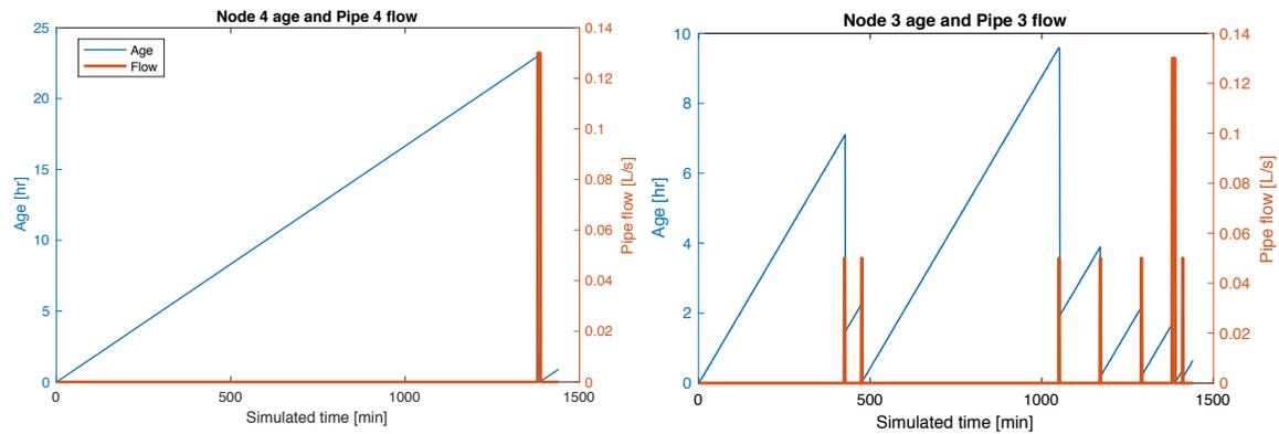
Figure 8: Age and flows obtained using PRVs at the dead-end pipes
