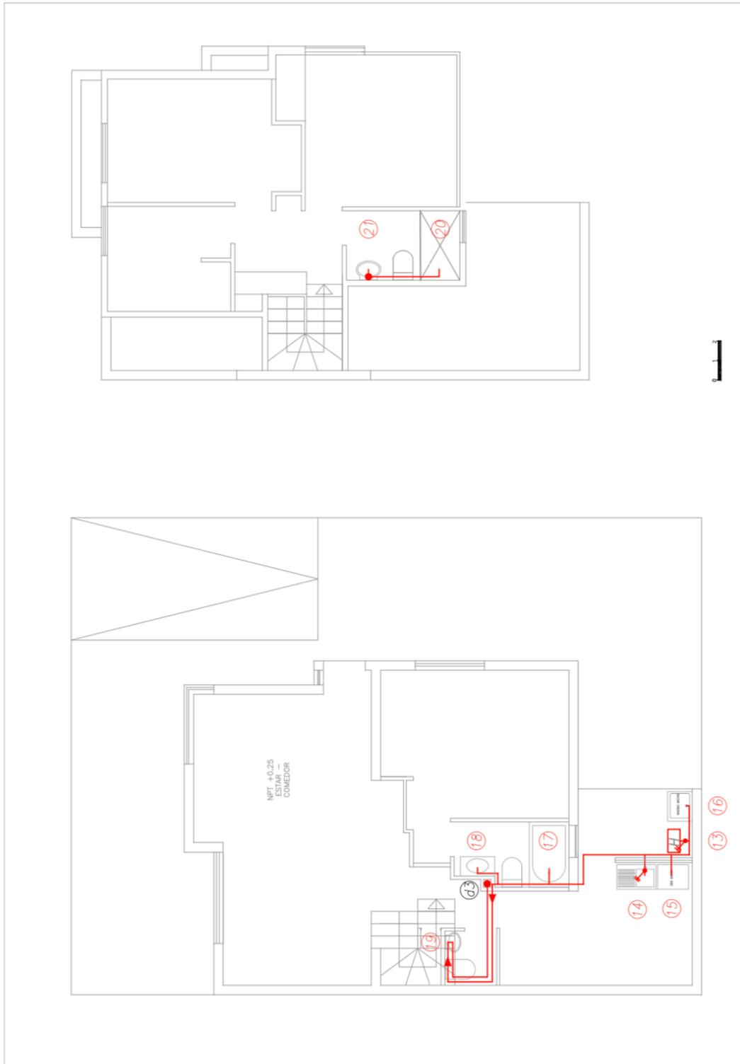
Figure A-6: house 1, layout 3 for the hot system
