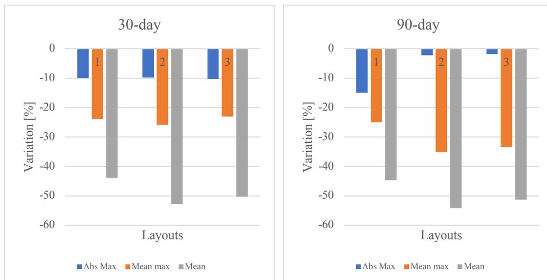
Figure 25: house 2 hot water residence time variation, traditional versus instant heater, at premise's distribution pipe
