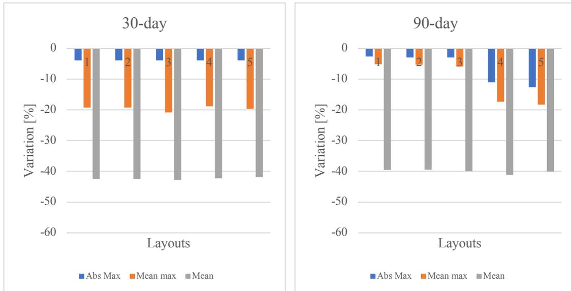
Figure 22: house 1 hot water residence time variation, traditional versus instant heater, at the node
