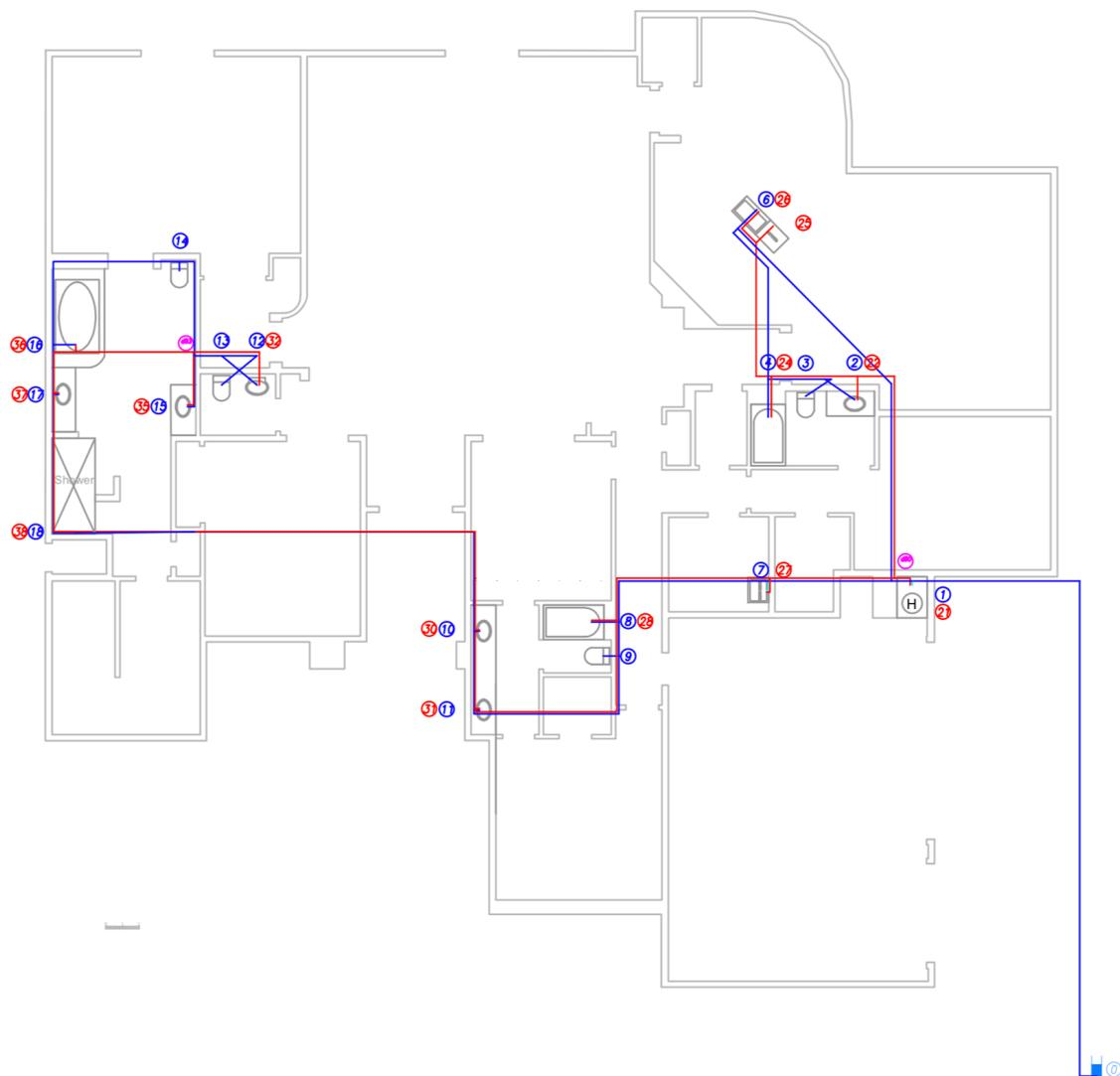
Figure A-12: house 2, layout 2 for both hot (red) and cold (blue) systems
