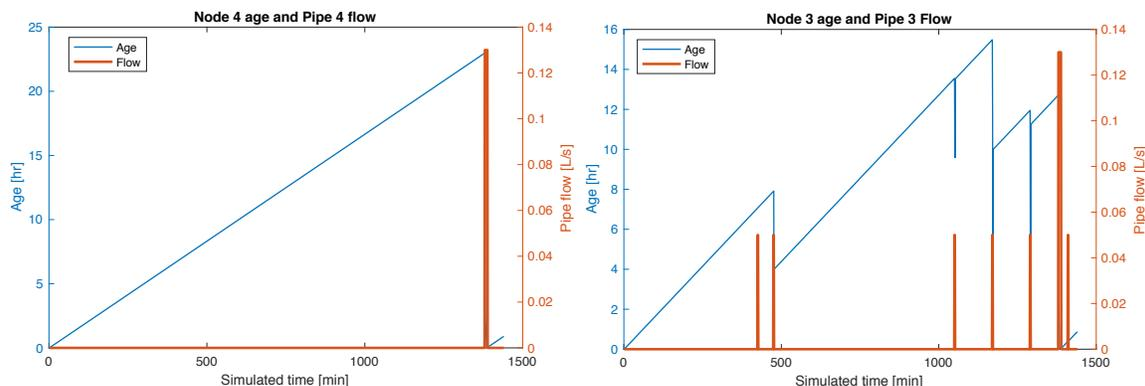
Figure 6: Age results when closing all pipes when downstream nodes have no demand
