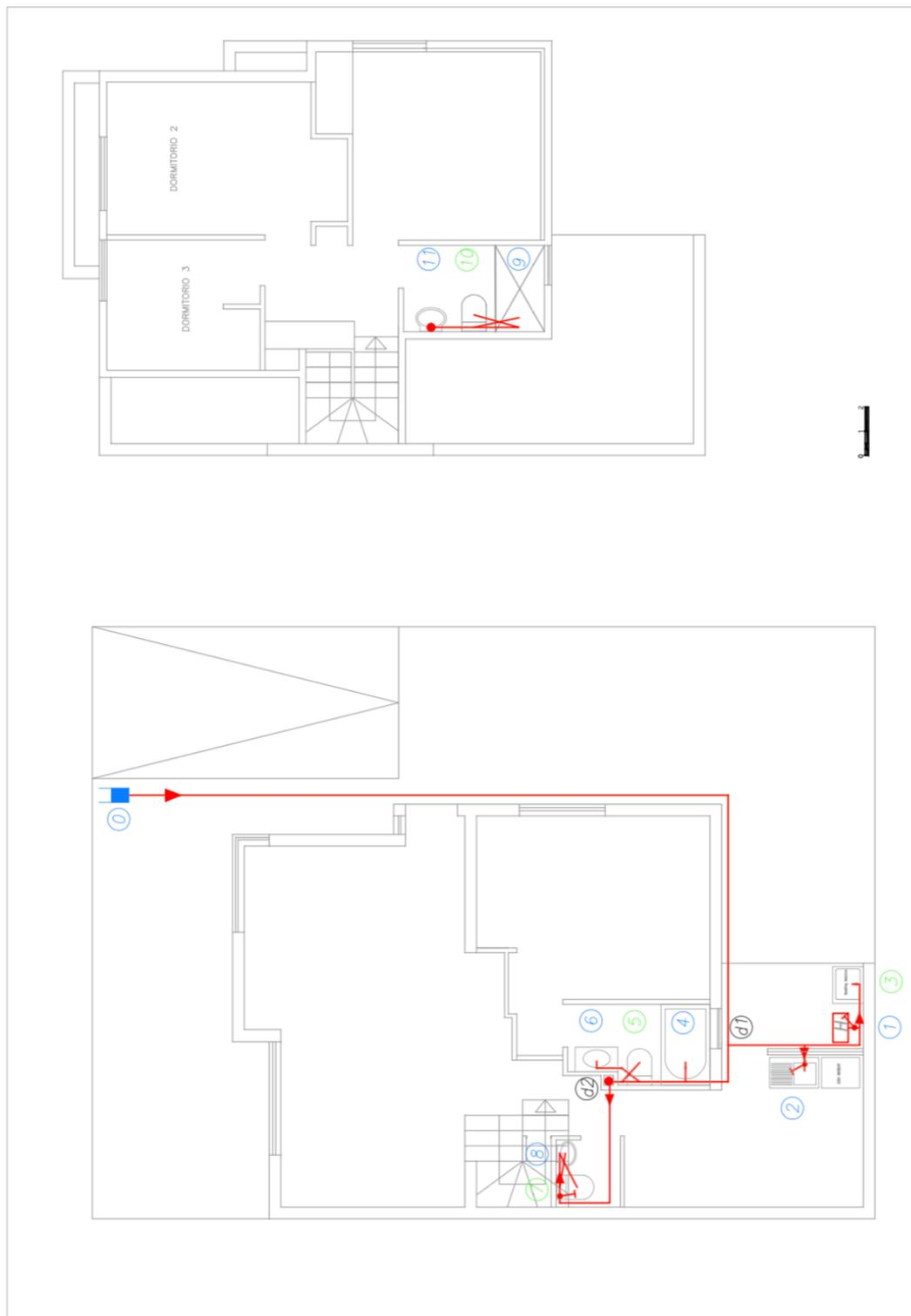
Figure A-3: house 1, layout 2 for the cold system
