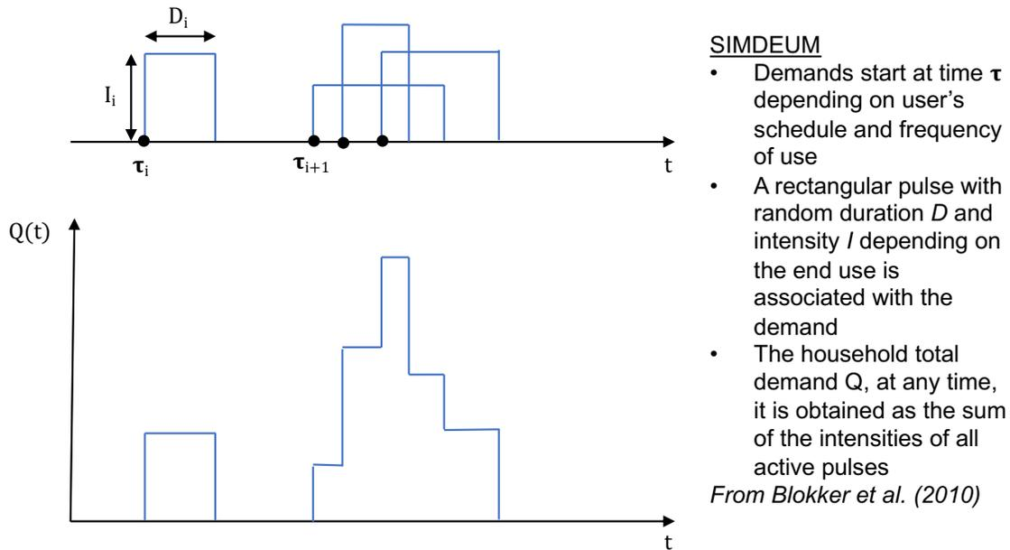
Figure 1: Schematic of residential demand characterization as rectangular pulses
