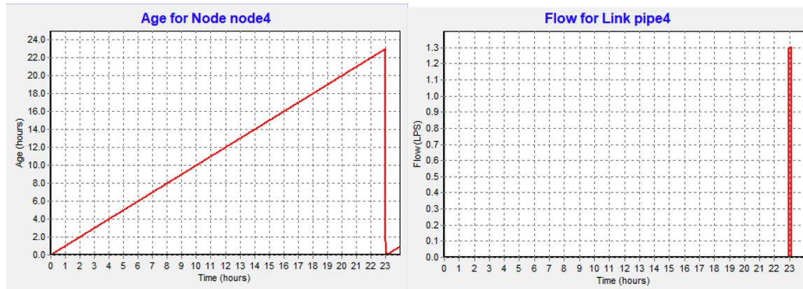
Figure 11: Age and pipe flow from EPANET, using the diameter factor approach
