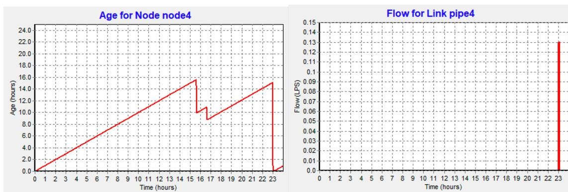
Figure 4: (left) Node 4 age time-series; (right) pipe flow time-series in the upstream pipe illustrating the demand
