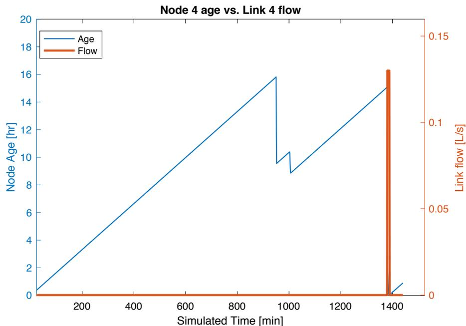
Figure 3: Time-series of water age in node 4, along with the upstream pipe flow illustrating the demand
