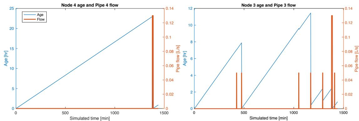
Figure 7: Age and flows obtained using PRVs at the start of each branch
