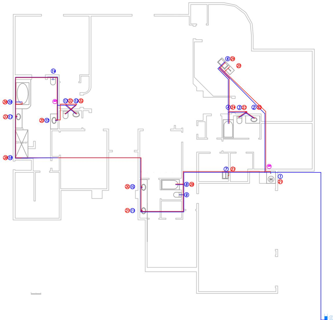
Figure A-14: house 2, layout 4 for both hot (red) and cold (blue) systems
