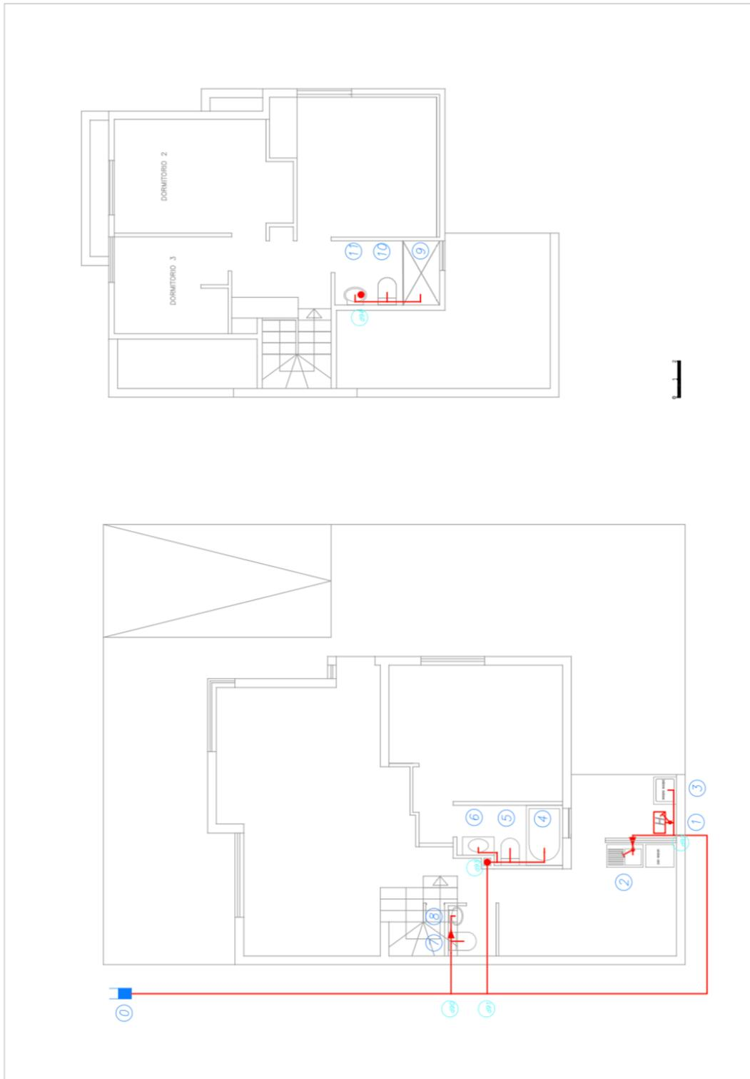
Figure A-7: house 1, layout 4 for the cold system
