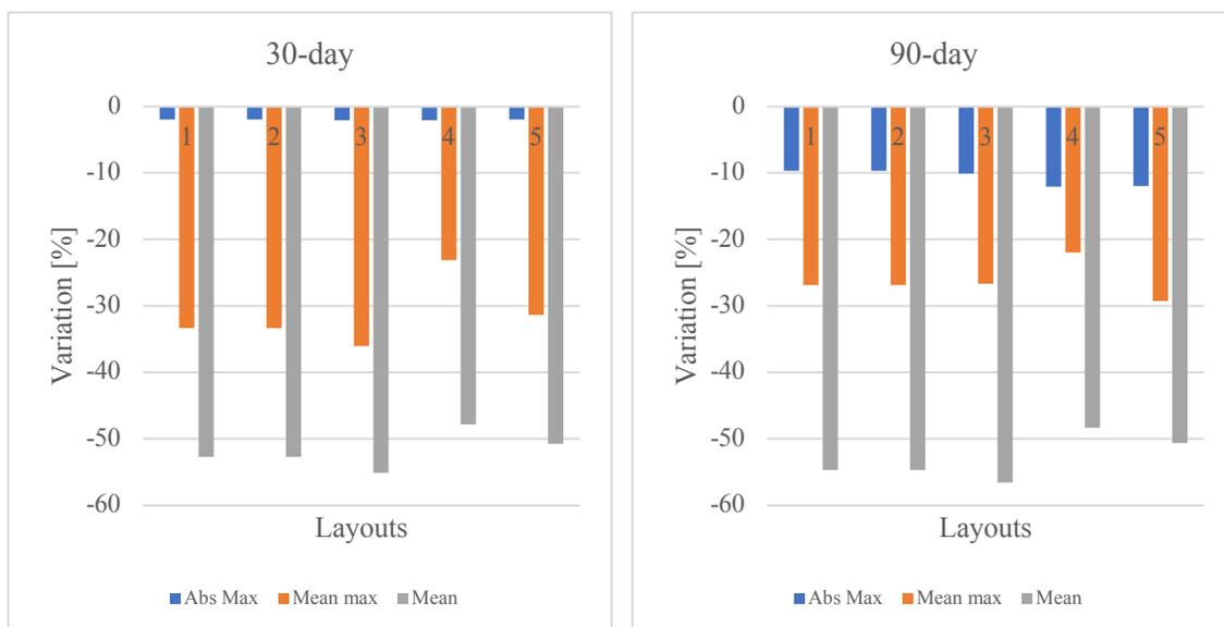
Figure 23: house 1 hot water residence time variation, traditional versus instant heater, at premise's distribution pipe
