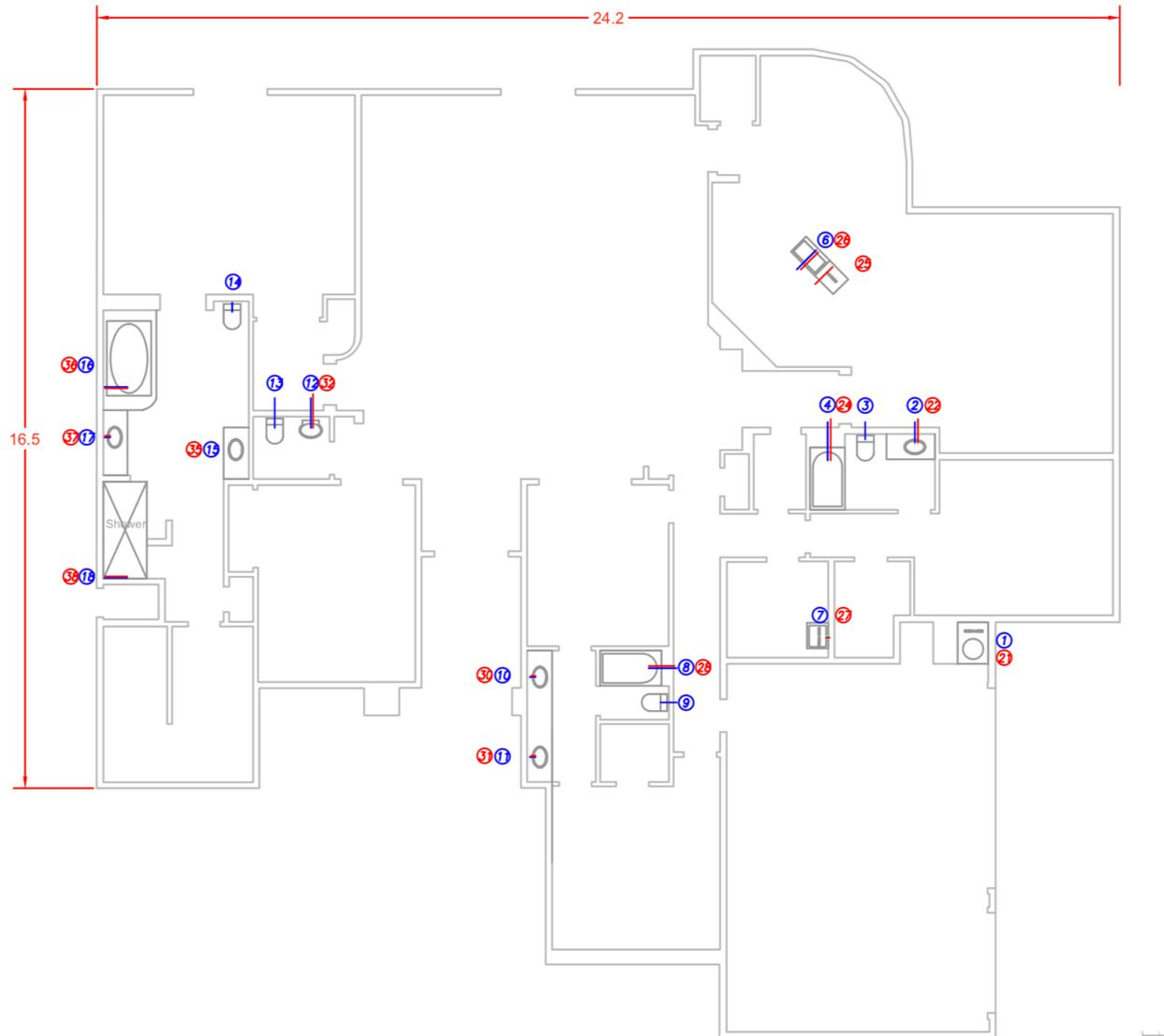
Figure 14: house 2 CAD plan, the blue circles are the nodes with cold water fixtures, while the red ones for hot water fixtures
