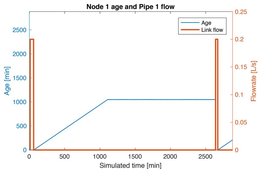
Figure 9: Age and flow for a sequential network comprised of 4 short pipes with long periods of no flow. Age plateaus in long periods of no demand, incorrectly.
