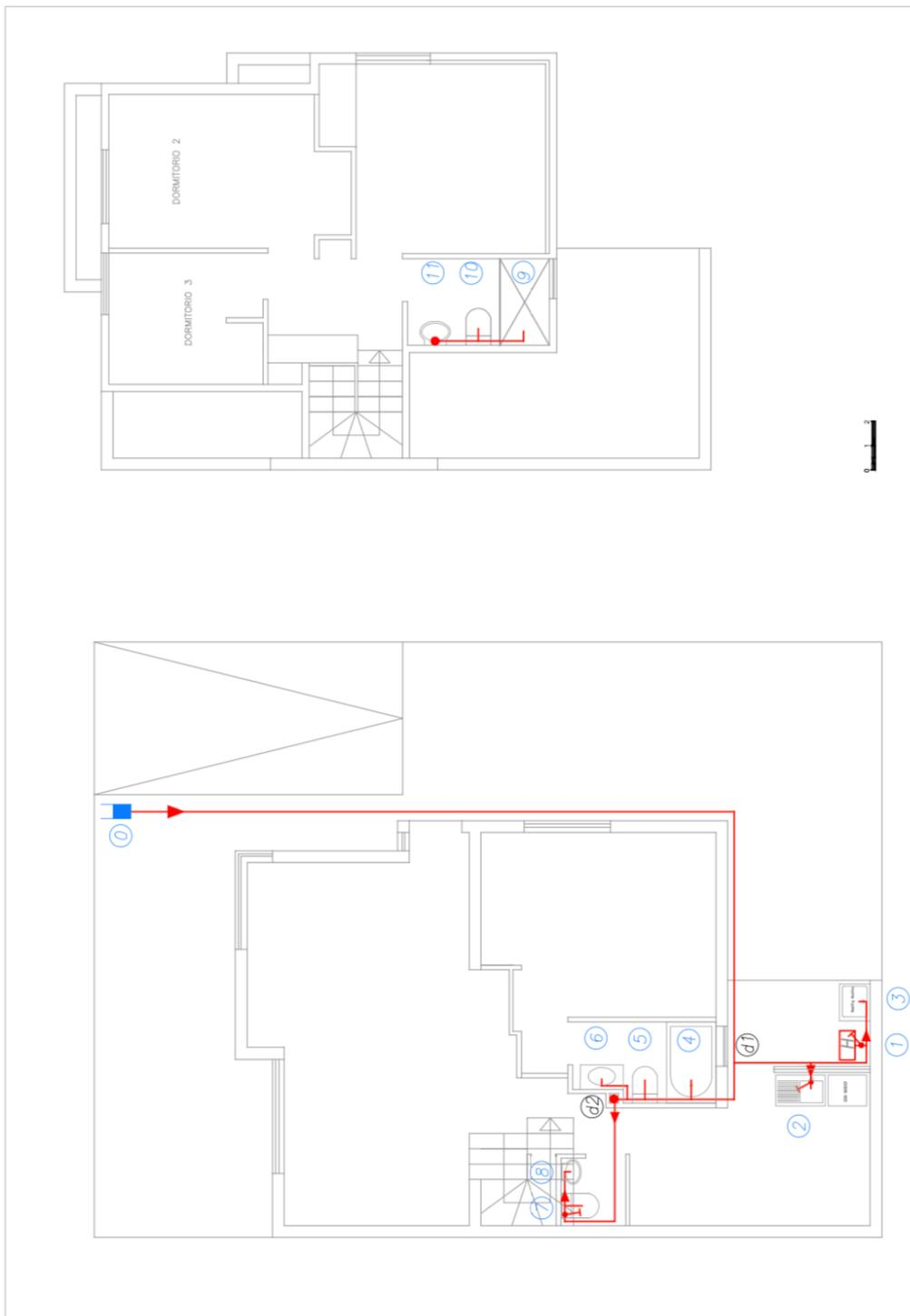
Figure A-1: house 1, layout 1 for the cold system
