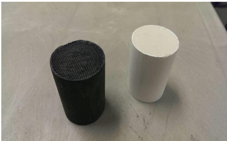
**Figure 8.** Picture of the Rh-NiO/La-K-Ce-Al-Ox/cordierite ATR catalyst (black) and support (white).
