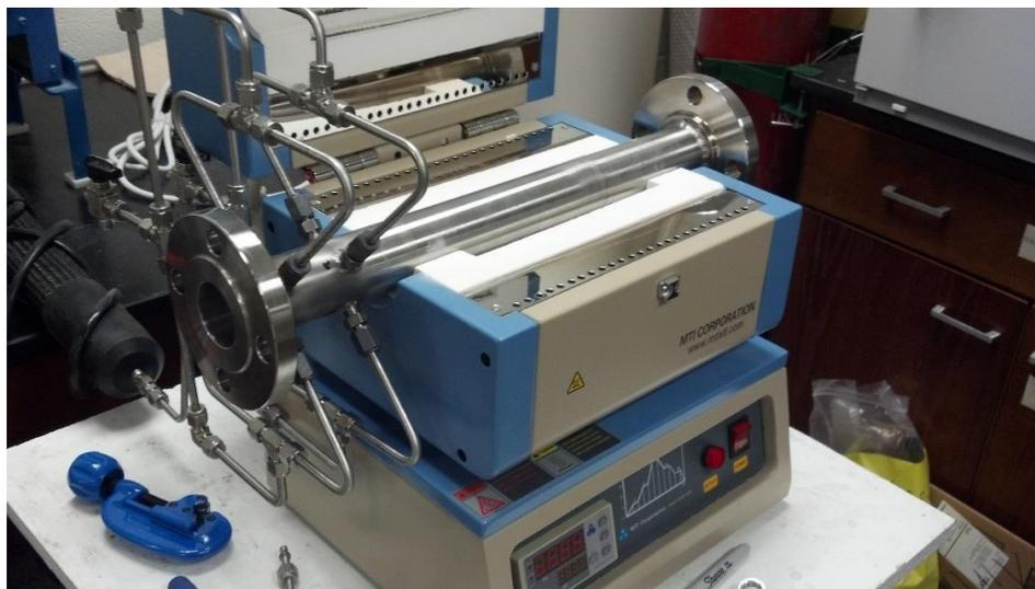
**Figure 10.** Previous version of ATR reactor without insulation.
