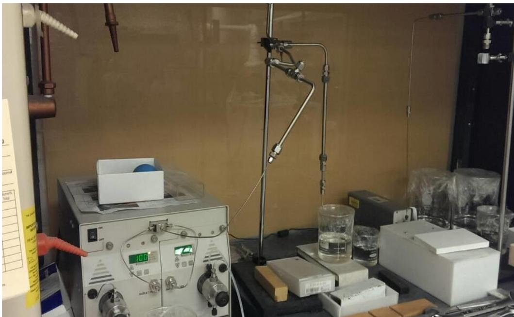
**Figure 6.** Adsorptive desulfurization test rig.
