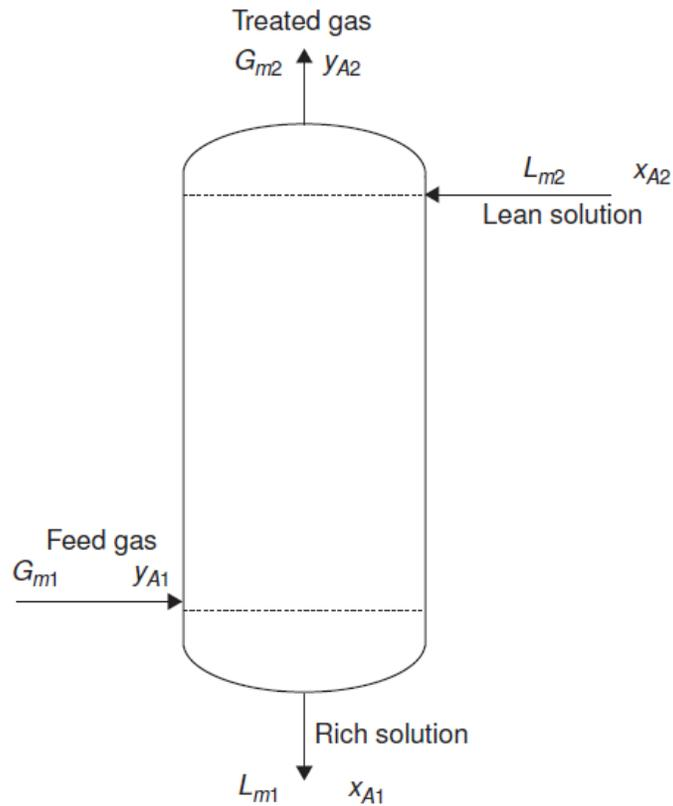
**Figure 10.7** Mole balance; countercurrent flow.
