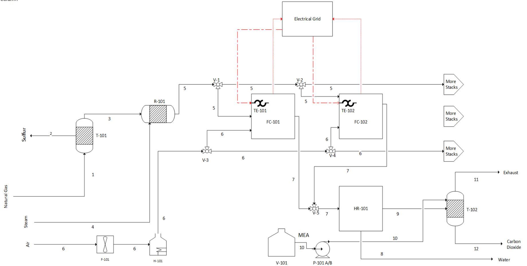
Figure 2: Process Flow Diagram
