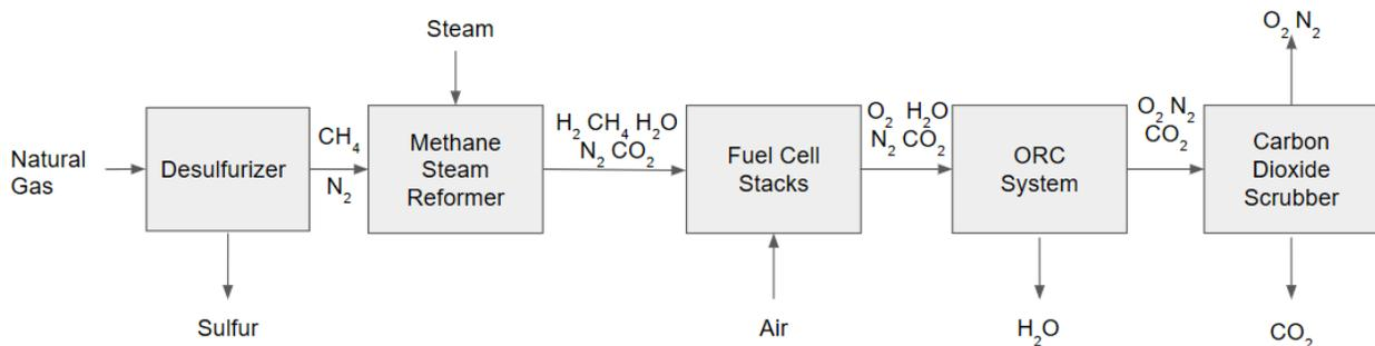
Figure 1: Block Flow Diagram
