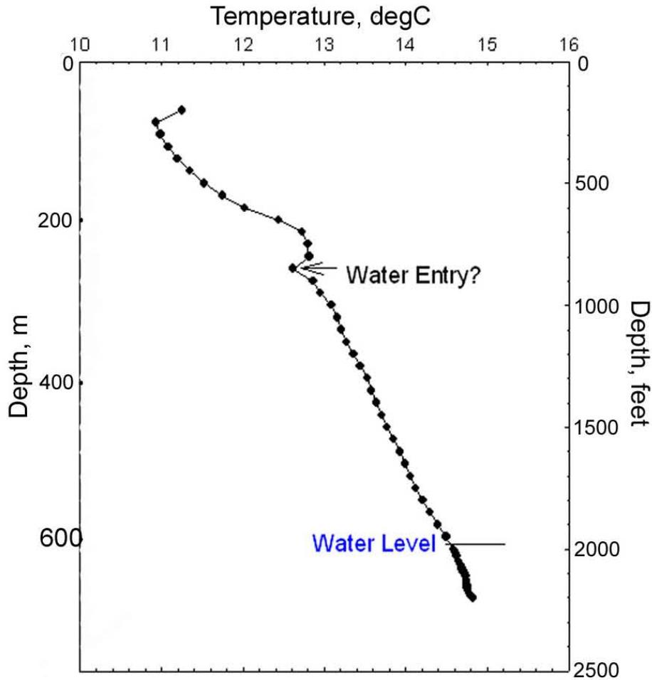
**Figure 10. Temperature Profile for SSC-1, near Sunset Crater**
