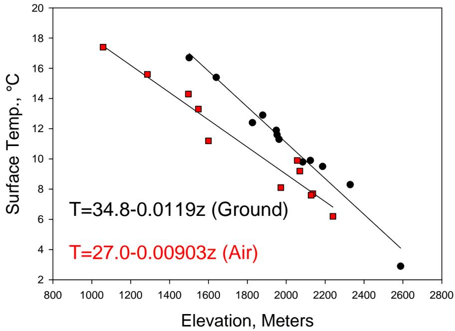
Figure 9. Air and Ground temperatures as a function of elevation for SFVF.
