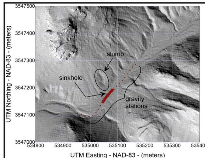
**Figure 1. Shaded relief map of the area within CCMP showing the locations of the sinkhole, the microgravity survey stations (in red) and a possibly related slump.**
