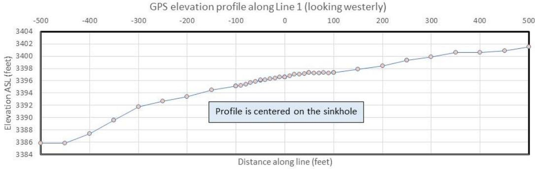
**Figure 6 Elevation profile of the full length of Line 1.**
