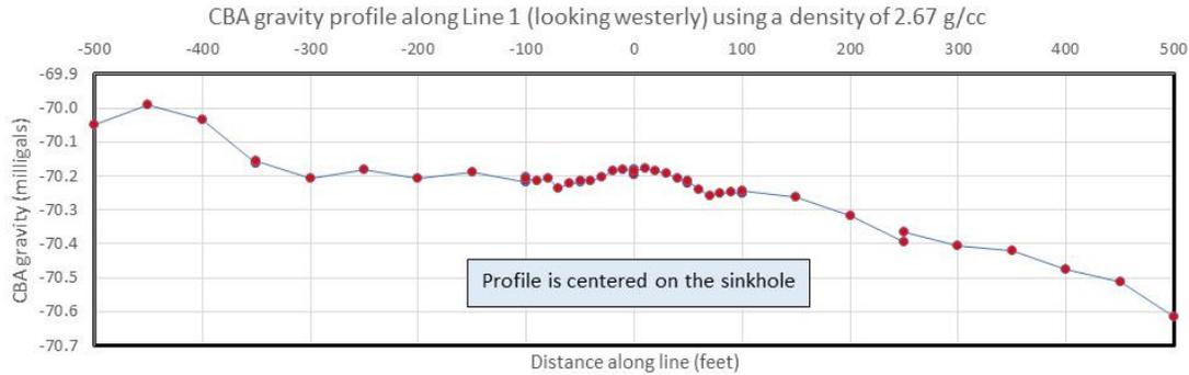
**Figure 8 CBA gravity profile for the full length of Line 1 (looking westerly).**
