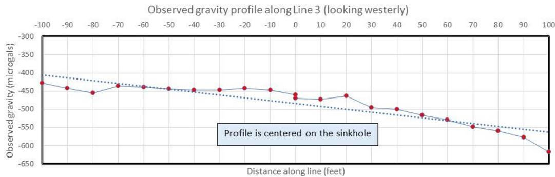
**Figure 5** Observed gravity for Line 3, looking westerly. The dotted line is a linear trend fit to the data for reference only.
