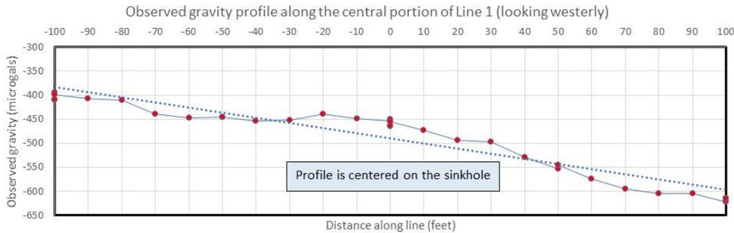
Figure 3 Observed gravity profile along the central portion of Line 1, looking westerly. The dotted line is a linear trend fit to the data for reference only.
