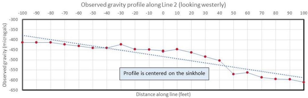
**Figure 4** Observed gravity for Line 2, looking westerly. The dotted line is a linear trend fit to the data for reference only.
