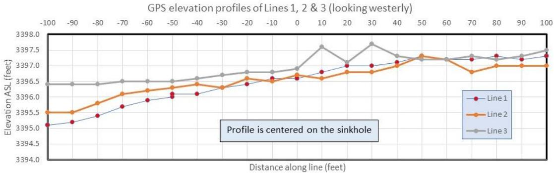
**Figure 7 GPS elevations of the three lines stacked for comparison. The lack of closer correspondence illustrates the lack of precision discussed in the text.**
