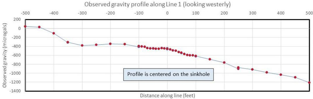
Figure 2 Observed gravity values for Line 1 full length, looking westerly.
