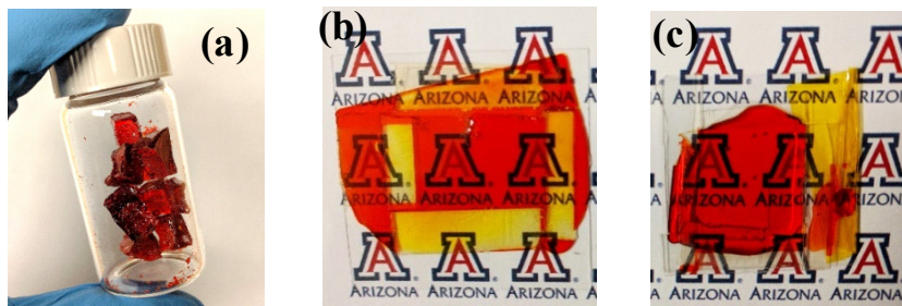
Fig. 1. Poly( S-r-DIB ) compounds: (a) Bulk sample of poly( S_{50\%} - r-DIB 50% ). (b) and (c) images through two thin samples of poly( S_{50\%} - r-DIB 50% ) and poly( S_{70\%} - r-DIB 30% ) with 291 \mu\text{m} and 415 \mu\text{m} thickness, respectively. Both materials have low transmission in the visible spectrum.
