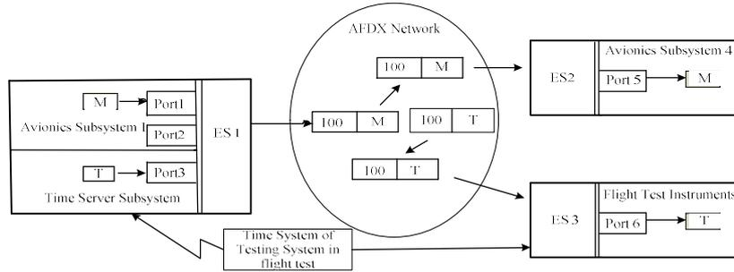
**Figure 5 Delay measurement of the AFDX time message**
