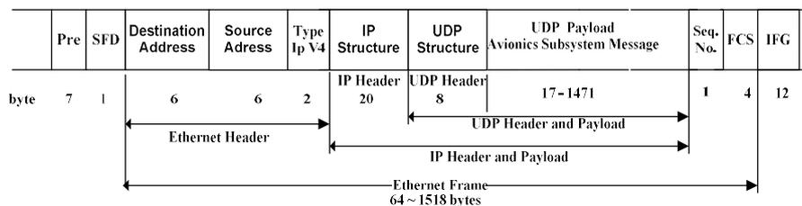
Figure 3 AFDX Frame Format
