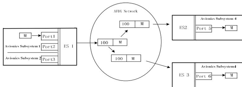
Figure 1 AFDX Message Processing Flow
