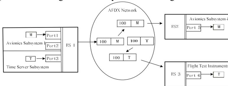
Figure 2 AFDX Flight Test Instruments
