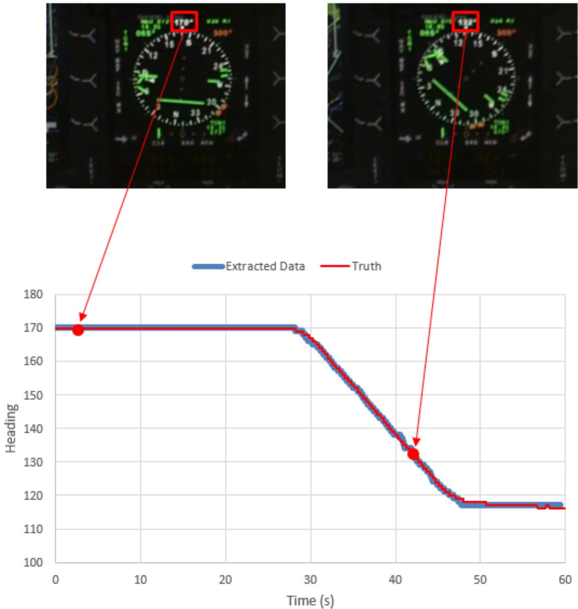
Figure 1. Measurements extracted from video processing compared to truth data (video courtesy Airbus Helicopters).
