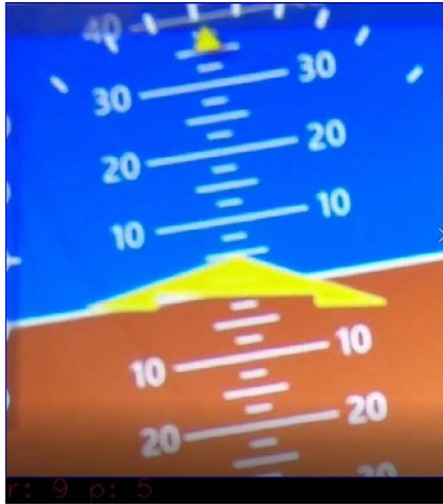
**Figure 2. Attitude indicator region of interest with roll and pitch extracted from video image shown at bottom of region.**
