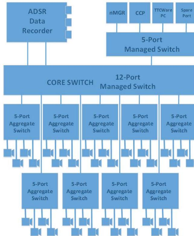
**Figure 1: High-speed cameras are often connected into larger networks to capture events from multiple angles**
