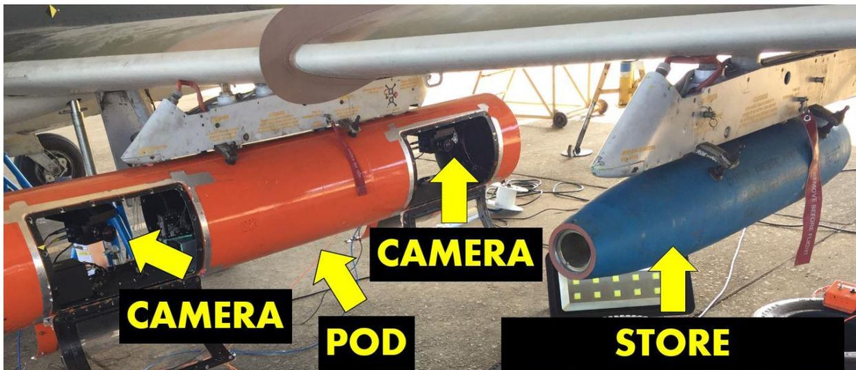
Figure 1 - POD used with two high-speed cameras.
