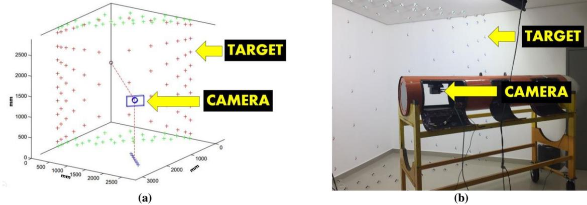
Figure 3 – IPEV Geometric Calibration Field. (a) Position of each simulated target in order to be homogeneously distributed in the captured image (b) Example of calibration of the rear camera.
