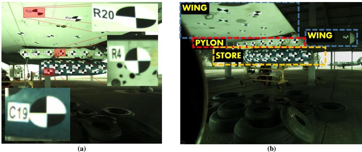
Figure 2 – Image example of front camera and rear camera. (a) view of the region of interest of the rear camera with zoom in 3 targets (b) frontal camera showing the ROI and the overview of the targets.
