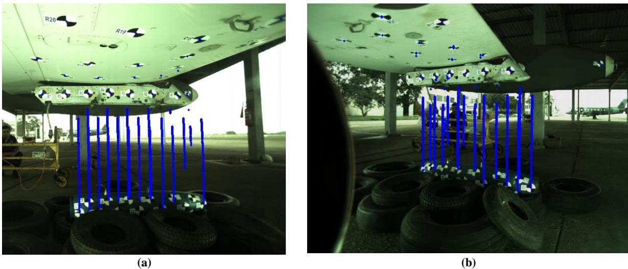
Figure 5 – Target tracking during test point (a) rear camera (b) front camera
