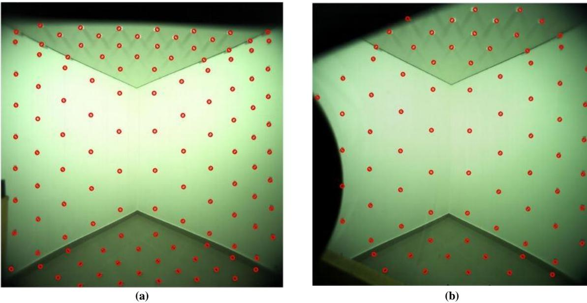
Figure 4 – Redesigned image of calibration field (a) rear camera (b) front camera.
