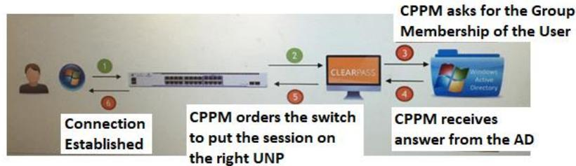
**Figure 6: Communication between Clearpass and Active Directory**
