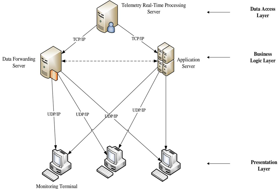
**Figure 6 Real-Time Monitoring System.**
