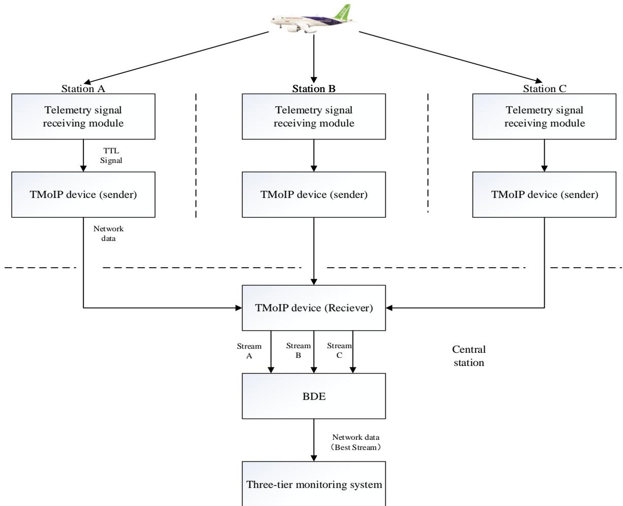
**Figure 1 System Architecture.**
