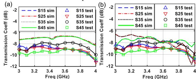
Fig. 3. (a) Measured and simulated transmission coefficients of the power divider. (b) Simulated transmission coefficients of the modified power divider model.
