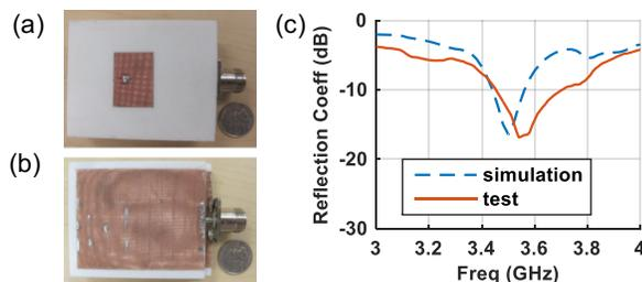
Fig. 7. Image of the (a) top view and (b) bottom view of the printed patch antenna with an N-type connector; (c) comparison of the simulated and measured reflection coefficients of the patch antenna.
