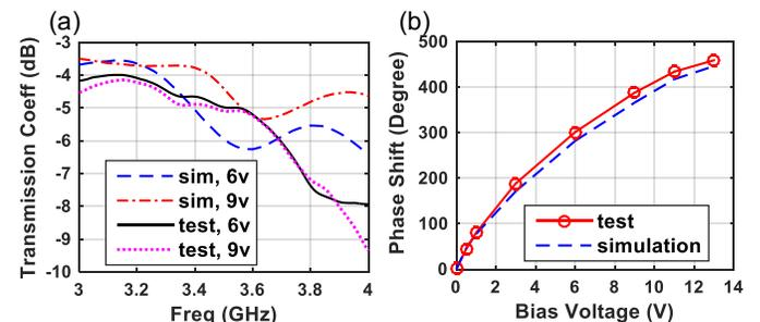
Fig. 5. Comparison of the simulated and measured (a) transmission coefficients and (b) the normalized phase shift vs. bias voltage at 3.5 GHz, of the phase shifter structure.
