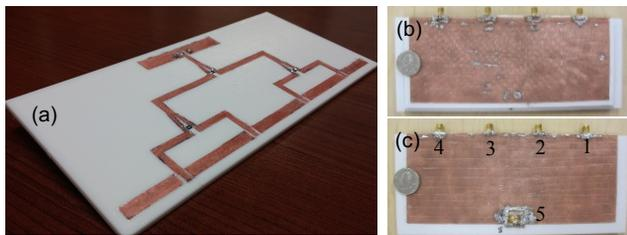
Fig. 2. Image of the printed 1-4 Wilkinson power divider: (a) without the top substrate and ground, (b) top view and (c) bottom view of the completed divider with SMA connectors.
