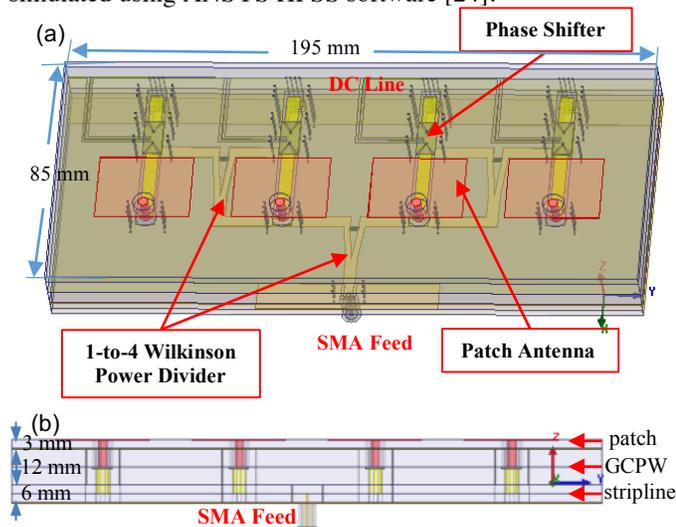
Fig. 1. Geometry of the designed 3D printable multilayer phased array: (a) perspective view and (b) side view.
