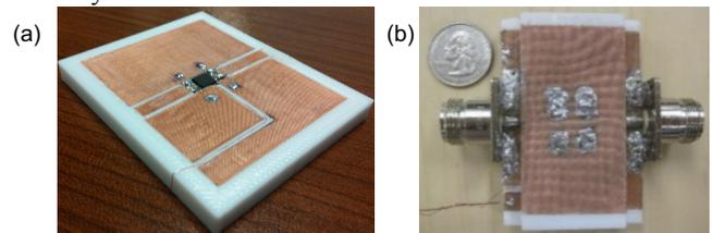
Fig. 4. Image of the printed phase shifter structure: (a) without the top substrate and ground, (b) top view of the completed structure with N-type connectors.
