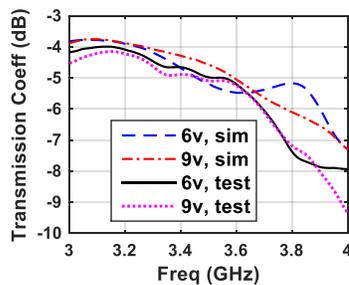
Fig. 6. Transmission coefficient of the phase shift layer from the measurement and the simulation of the modified-model.
