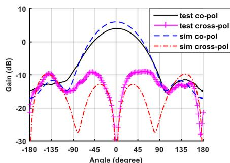
Fig. 8. Comparison of the simulated and measured antenna gain of the patch antenna at 3.5 GHz.
