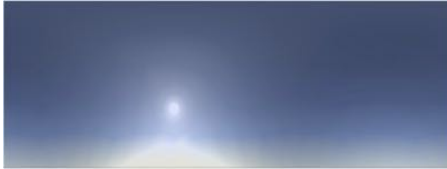
Figure 6: Output of MODTRAN diffuse sky radiance, arranged as a sky map suitable for input to the Mitsuba rendering software.
