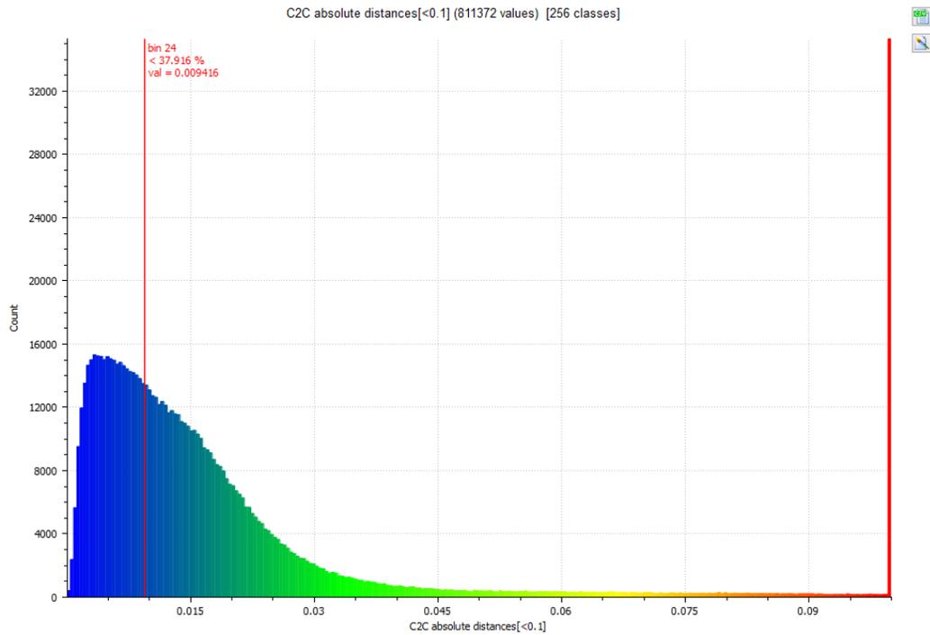
Figure 28 Histogram showing the distribution of point cloud scalar color after performing change detection.
