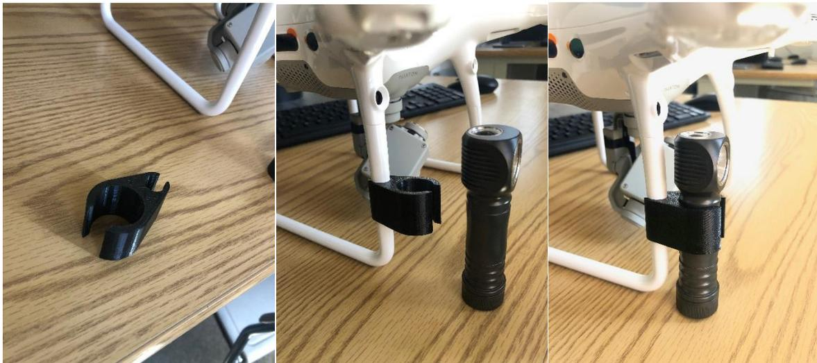
**Figure 17 Clamp designed in Solidworks and manufactured in 3D printer to mount Zebralights on the Drone**
