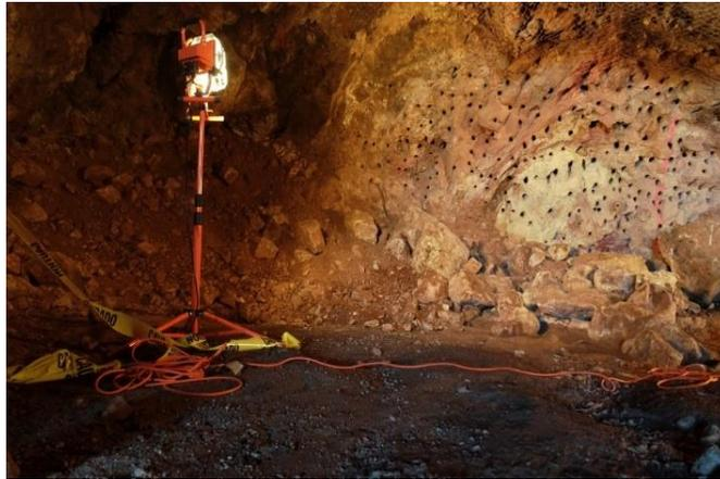
Figure 20 The setup of halogen lights for flight test 6
