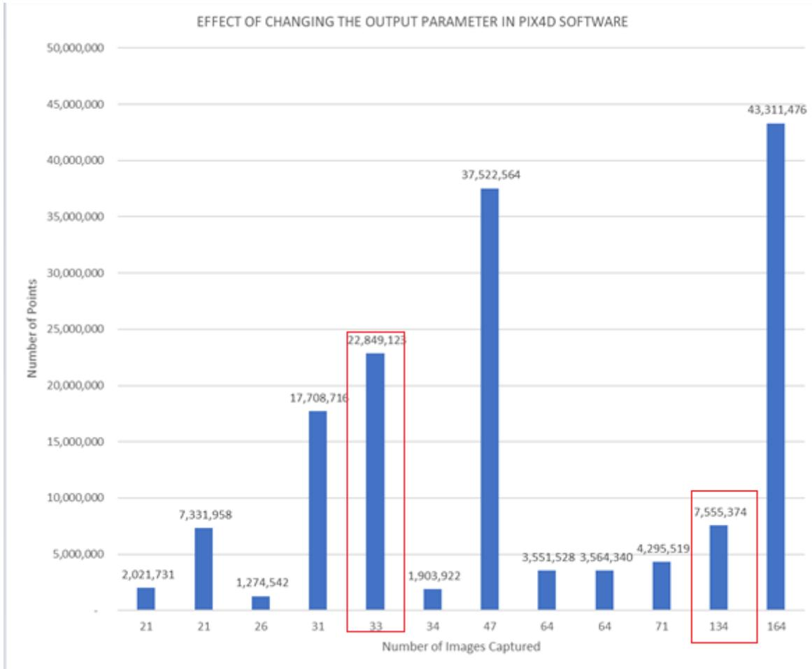
Graph 3: This graph demonstrates the effect of changing the output parameter in the PIX4D software like point density and image scale can change the total number of points generated.
