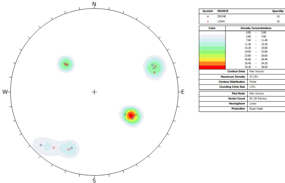
Figure 29 Stereonet projection of 20 different planes generated by Drone and LIDAR point cloud
