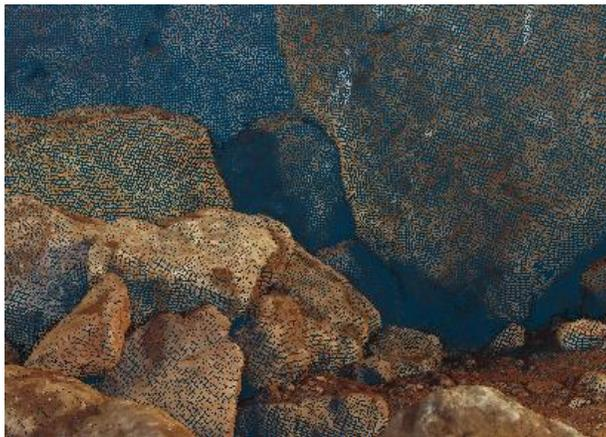
Figure 21 Voids in the point cloud after test flight 6
