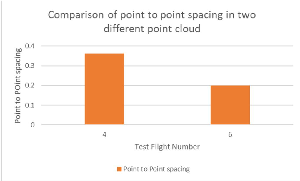
Graph 1: The spacing between two points in point cloud generated by test flight 4 and 6. (The value on Y axis is normalized value and not in feet or centimeter)
