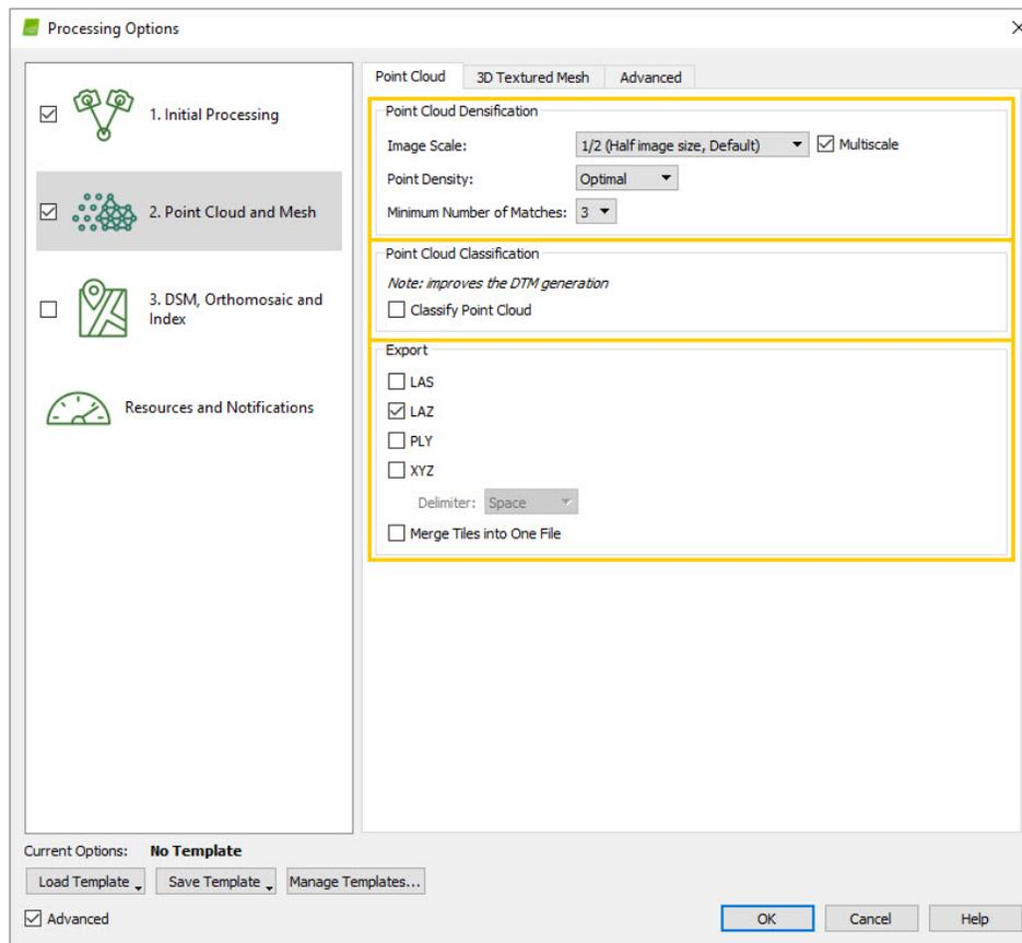
Figure 11 Options for changing the input to vary the output of the point cloud like density, image scale and the format of the output file
