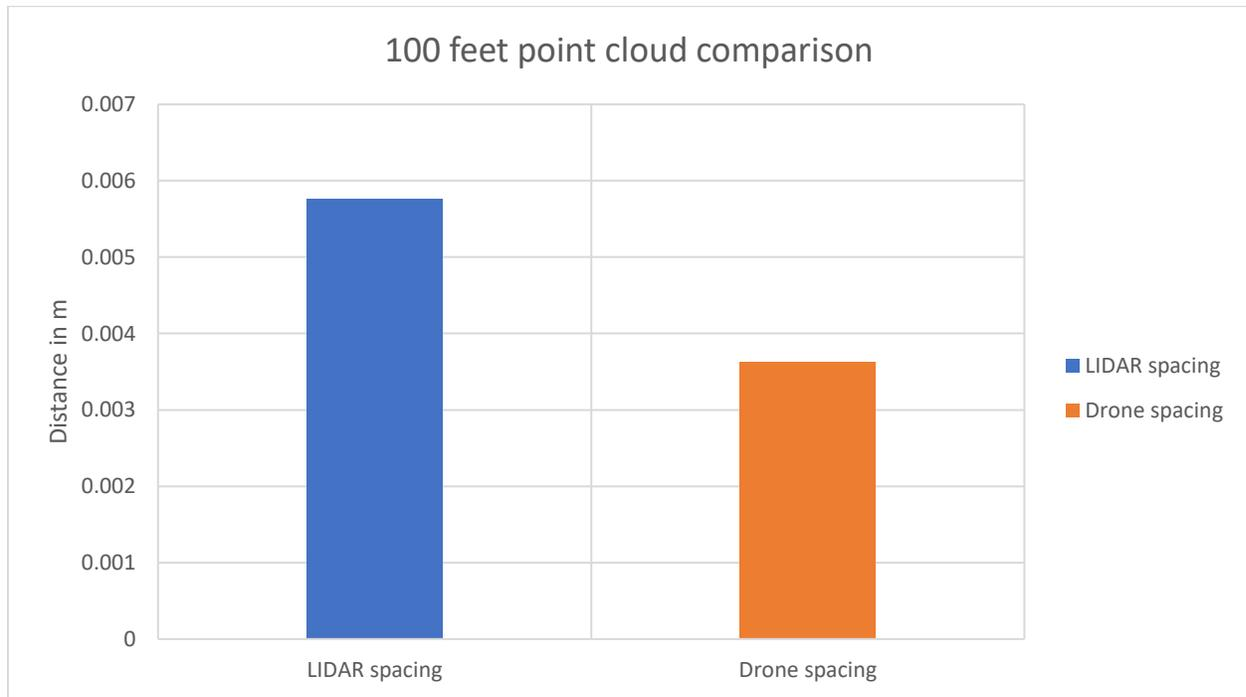
**Graph 4: Comparison of point spacing between point cloud from LIDAR scan 1 and test flight**
