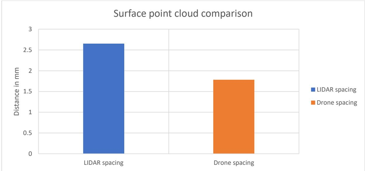
Graph 5: Comparison of point spacing between point cloud from LIDAR scan 2 and test flight 17
