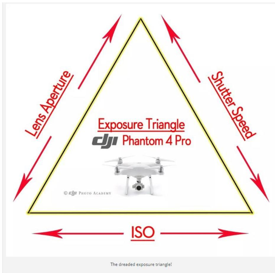
Figure 14 The Dreaded Exposure triangle shows the relation between lens aperture, shutter speed and ISO
