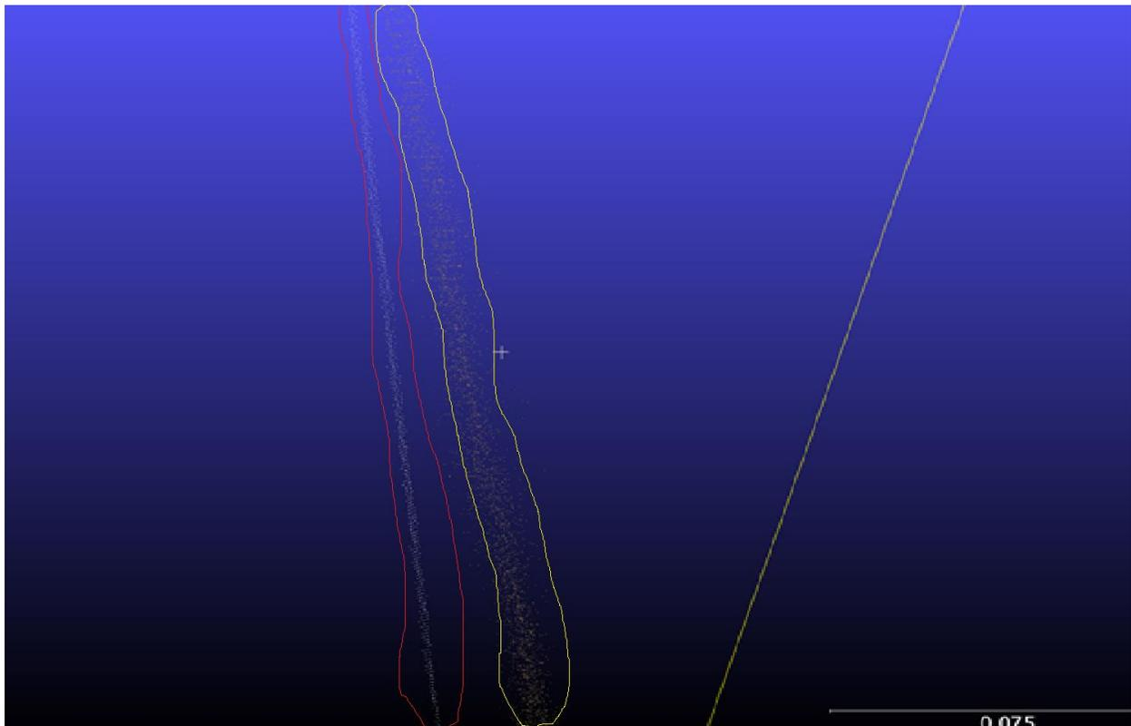
Figure 24 A comparison of the point cloud data of a flat surface for thickness. The red area is a point cloud from LIDAR and yellow is point cloud from the drone
