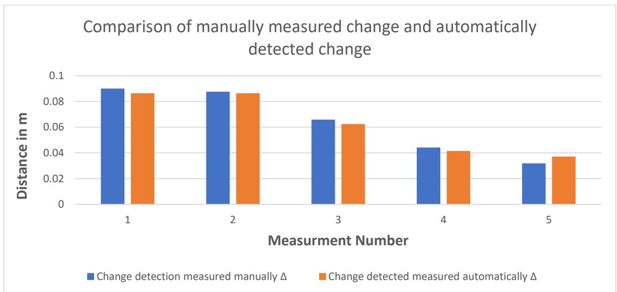
Graph 6: Comparison of the change detection measured manually and automatically using the cloud to cloud distance
