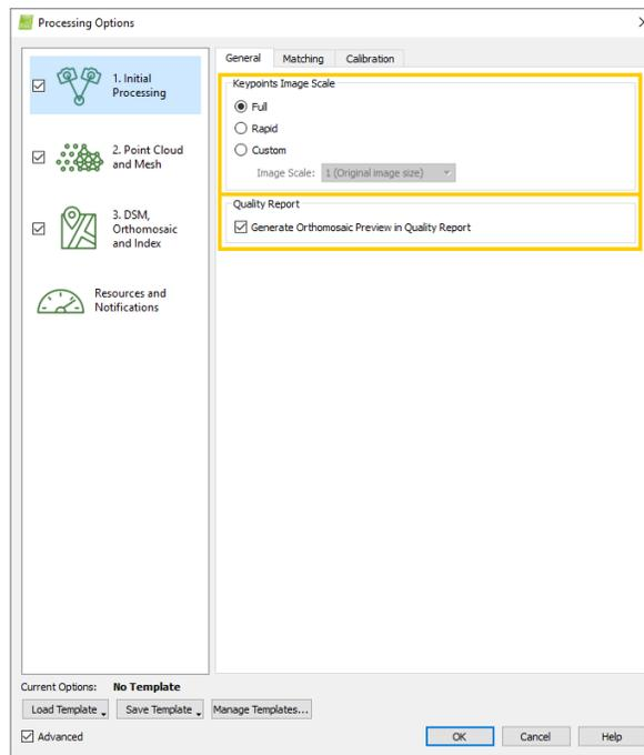
Figure 10 Initial processing option in PIX4D software
