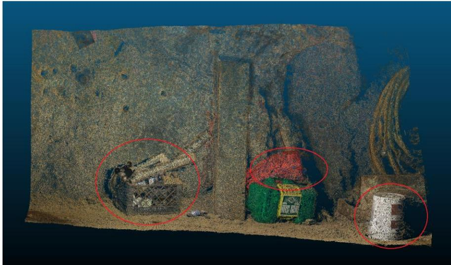
Figure 26 Drone point cloud from test flight 11 at 100 feet level at the SX Mine. The red circle shows the object that is not present in the LIDAR point cloud
