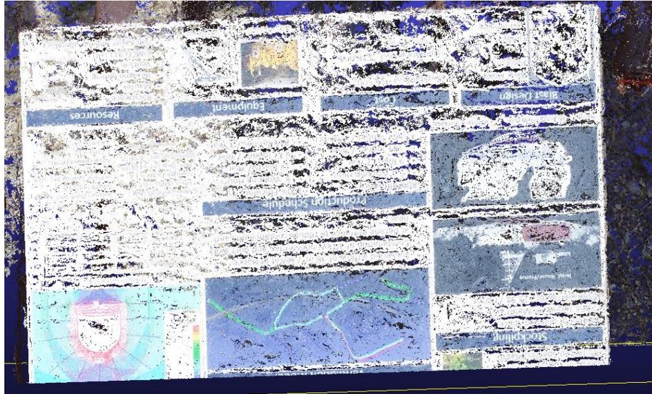
Figure 23 Noise generated after scanning a piece of flat surface. The white portion has significant amount of noise as compared to other section with texts
