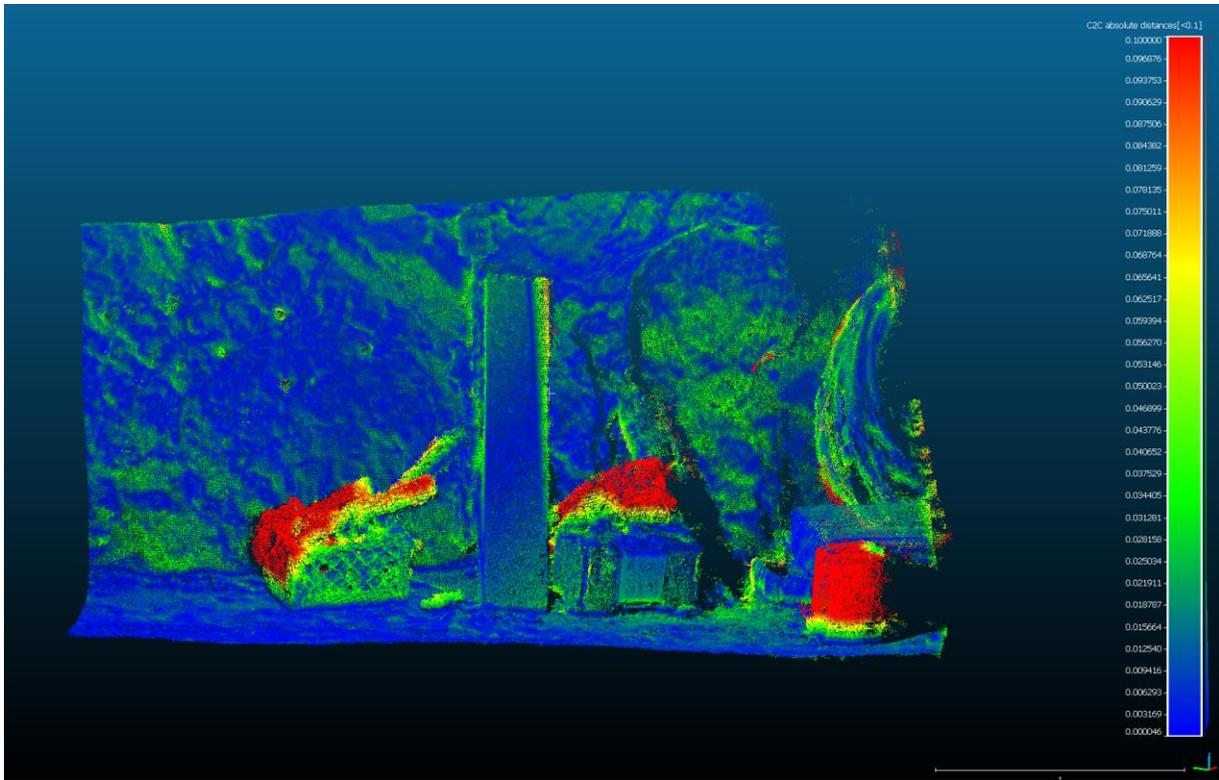
Figure 27 The result after performing change detection between test flight 11 and LIDAR scan 1
