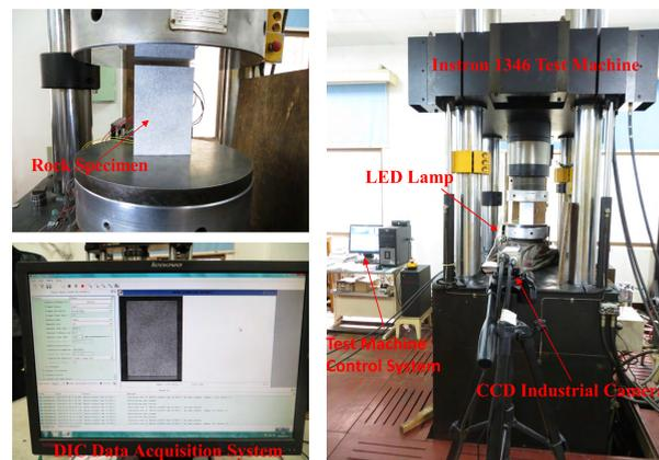
**FIGURE 5.** Uniaxial compression test system for specimens.
