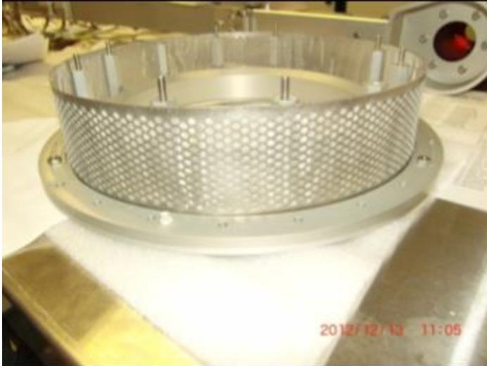
The “wall” of TAGSAM sample volume consists of two layers:
