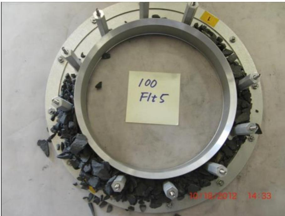
Test collected 325.4 g, photo is collected material Initial contact slightly presses large rocks into the regolith. Gas firing excavates smaller material at depth, and larger rocks are pushed further down, allowing TAGSAM access to more of the bulk regolith.
