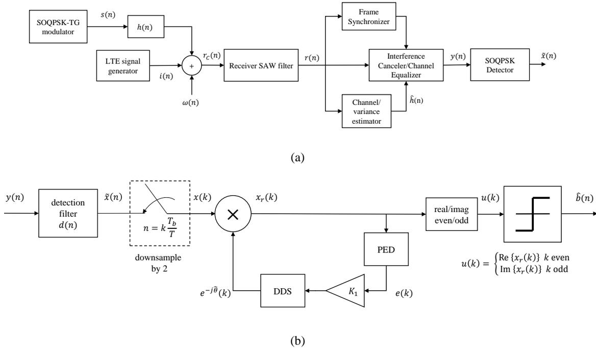
Figure 2: Block diagram: (a) Telemetry system in the presence of LTE interference, (b) SOQPSK detector.
