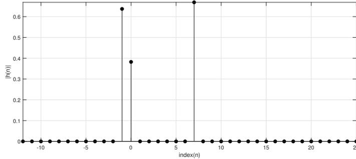
Figure 4: Telemetry multipath channel.
