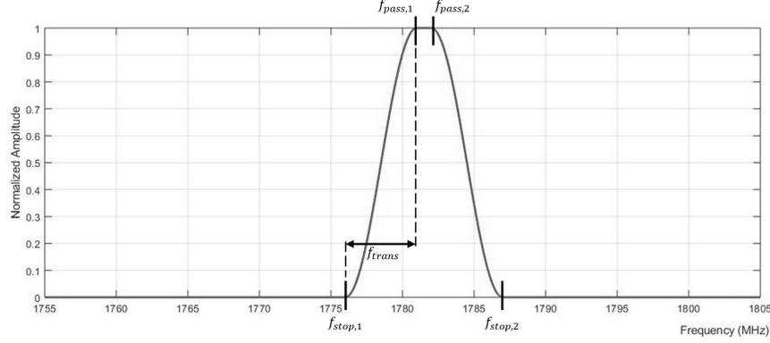
Figure 3: Digital IF SAW filter at AMT receiver with center frequency at 1781.5 MHz,  $f_{stop,1} = 1776$  MHz,  $f_{pass,1} = 1781$  MHz,  $f_{pass,2} = 1782$  MHz,  $f_{stop,2} = 1787$  MHz,  $f_{trans} = 5$  MHz.
