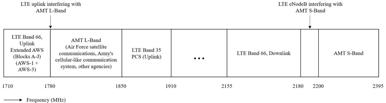
Figure 1: AWS-3 and telemetry adjacent bands.
