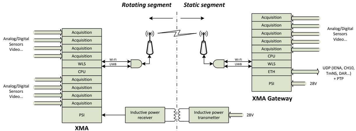
6 Global installation for data and energy transmission on a rotor
