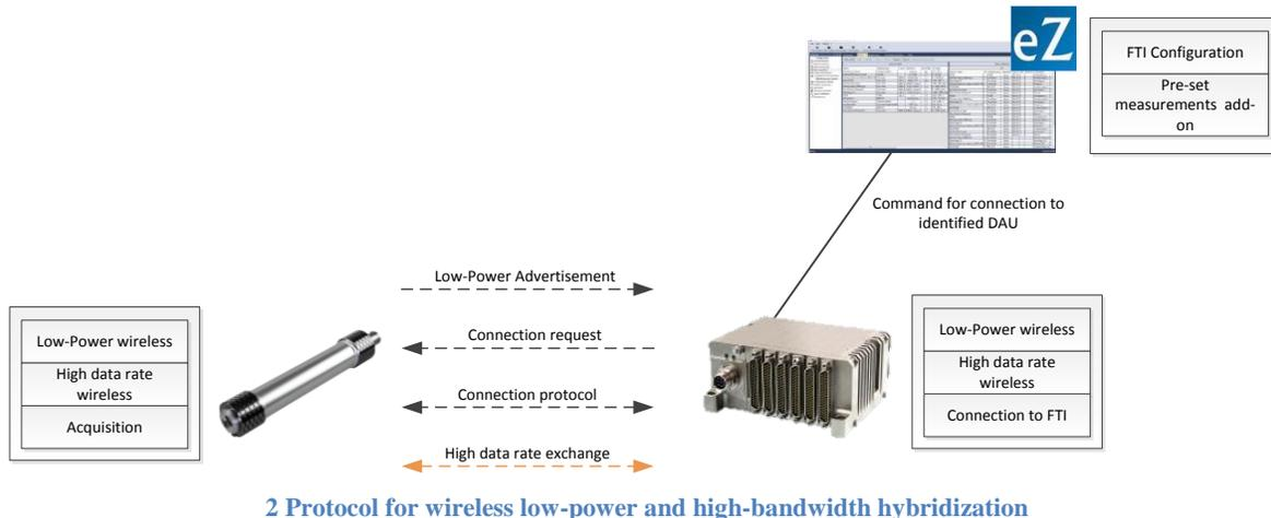
Such protocol enables to quickly add new measurements with equipment that can be battery-powered, staying at low levels of power consumption while permanently available for connection.
