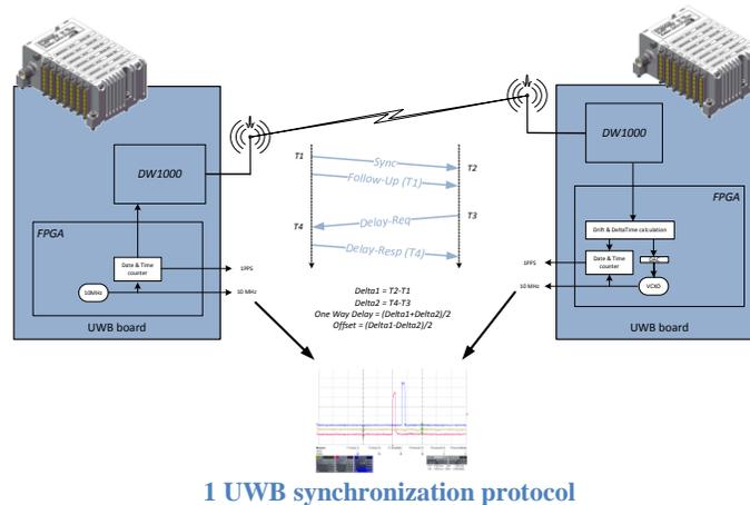
The synchronization architecture is based on a DAC and a VCXO enabling phase and phase clock alignment. This solution was tested and <10ns of synchronization accuracy was reached. Integration of this wireless link in a standard instrumentation architecture safeguards a <100ns accuracy throughout the system (inducing a <1° phase accuracy between two 20kHz signals, equivalent to signals acquisition in the same DAU).
