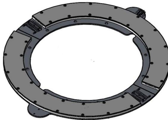
**5 Mechanical housing of stator for inductive power transmission**
