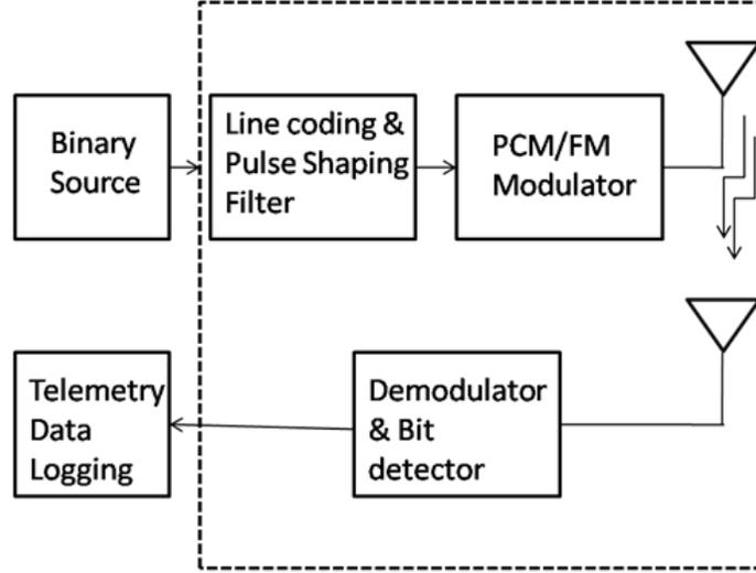
Figure 3: Block Diagram of the System Model
