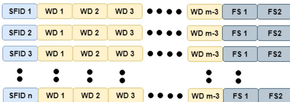
Figure 2: IRIG-106 Telemetry PCM Frame format
