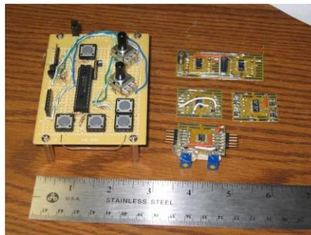
**Figure 3 Second prototype system for the ultrasound navigation system.**
