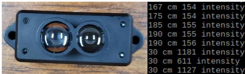
Figure 8 TFMini Module and Range Information Displayed in Terminal.
