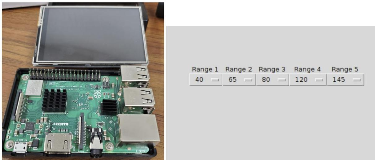
**Figure 9 Raspberry-Pi and Touch Screen Module with User Interface.**
