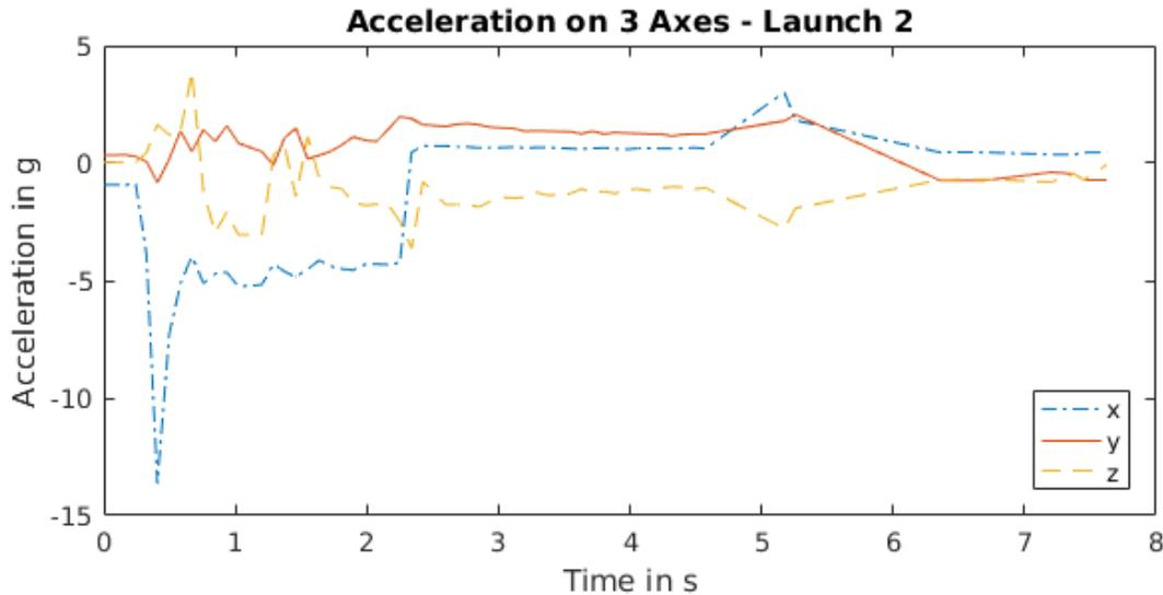
Fig. 3: Measured acceleration versus time graph of second flight. Launch occurs at 0.2 s with the engine shutting off at 2.4 s. The parachute charge is fired at 4.7 s, and takes effect at 5.3 s.
