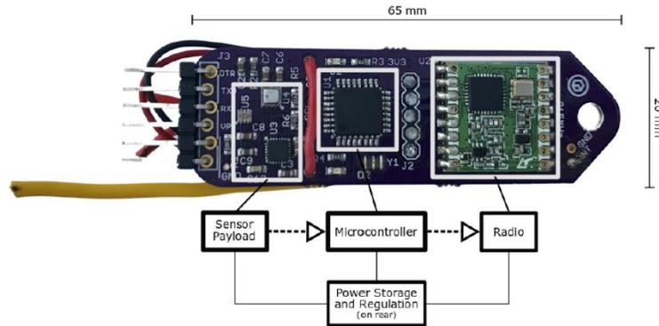
Fig. 1: Hardware photograph of a typical femtosat showing the key components. Power comes from a backside-mounted battery. The yellow wire at left is the antenna.
