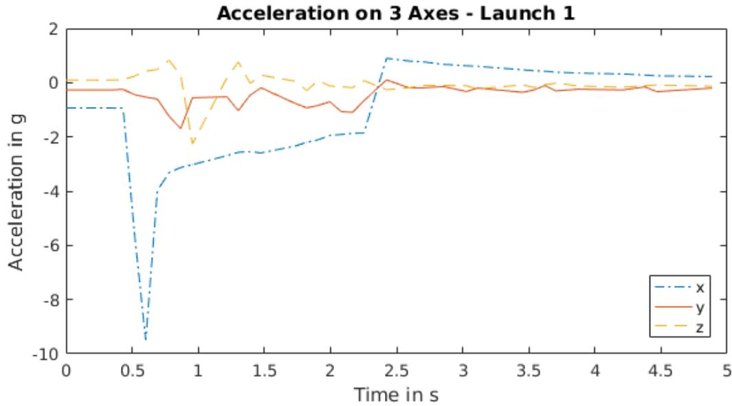
Fig. 2: Measured acceleration versus time for a particular flight. Launch occurs at approximately 0.5 s, with the engine shutting off at 2.3 s. Launch impact on the ground occurs 30 s later (off the plot).
