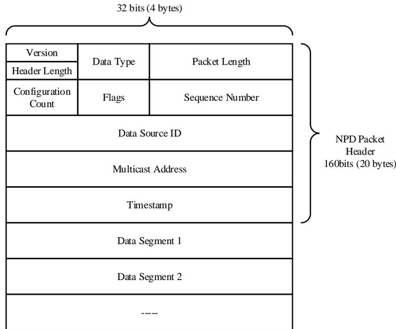
**Figure 1 NPD data packet.**
