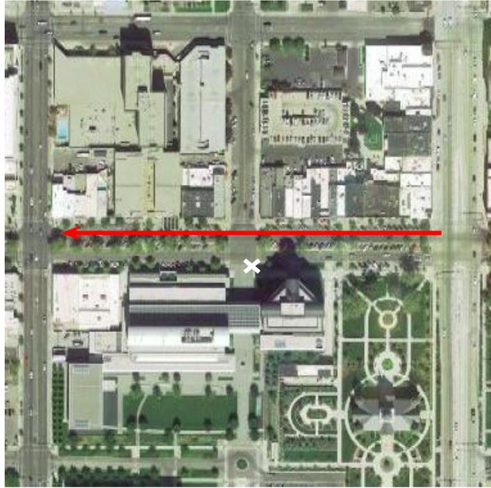
Figure 3: Routes for the channel measurement test points. V2I measurements were collected by parking the van with the transmit antenna at the location marked with a white “x”, while the red arrow marks the route followed for both V2I and V2V measurements. For each V2V test point the vehicles followed the same route but with varying degrees of separation between one another.
