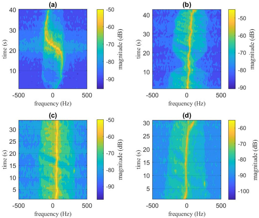
Figure 4: Top view of the gain in the channel with respect to time. Yellow corresponds to a higher gain, while blue corresponds to a lower gain that approaches zero. Four test points were measured and correspond to (a), (b), (c), and (d).
