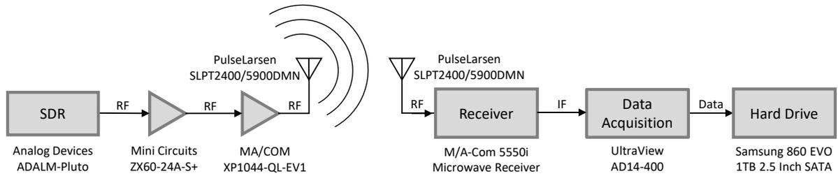
Figure 1: Block diagram of system setup.
