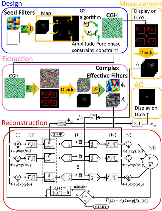
Fig. 2. Algorithm of single-shot phase retrieval with the complex diversity, and AO correction.
