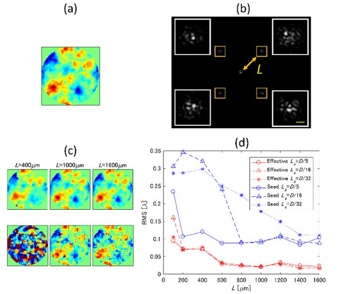
Fig. 3. Simulation results. (a) An extrinsic Kolmogorov aberration. (b) A simulated irradiance pattern at the image plane. The scalebar shows 100  $\mu\text{m}$ . (c) Retrieved aberrations with  $L_s = D/16$ . The effective filters (top) and the seed filters (bottom). (d) Residual RMS.
