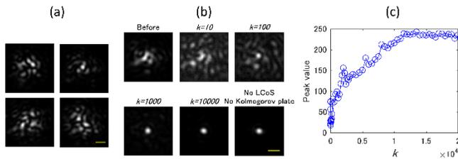
Fig. 4. Experimental results. (a) Four phasograms divided from a measured irradiance image. The scalebar shows  $100 \mu\text{m}$ . (b) AO correction results. The top left is the image before correction, and the bottom right is the image without the LCoS and the artificial Kolmogorov phase plate. The others show the images corrected with the estimated phases at the iteration  $k$ . The scalebar shows  $100 \mu\text{m}$ . (c) Peak values of the corrected spots.
