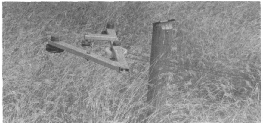
Fig. 3. Pulley apparatus which forms the union of the frontal fence and lateral line. Also shown is a lateral line post and wire guide.
