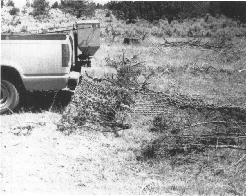
*Side view showing the action of the drag chains over woodcutting debris.*
