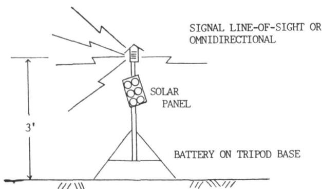
Fig. 1. Signal Transmitter/Receiver (STR)
