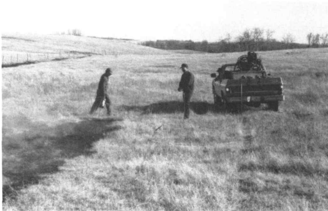
A slip-on fire suppression unit modified for rangeland burning. Photos by Barry Irving.
