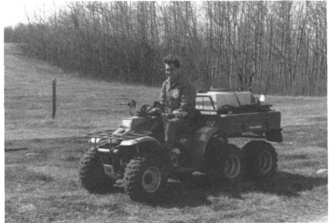
A 6-wheel all terrain vehicle fitted with fire suppression equipment. Photo by Barry Irving.
