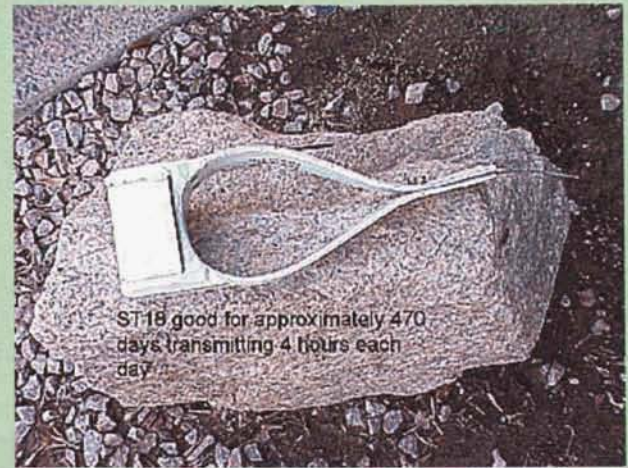
Figure a Collar with ST18 PTT and VHF in sealed canister. Note VHF antenna (non-insulated cable) and PTT antenna (insulated short black object between canister and end of collar). (Source: Telonics)
