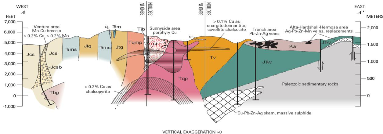
FIGURE 3B: GEOLOGIC CROSS-SECTION<sup>1</sup>
