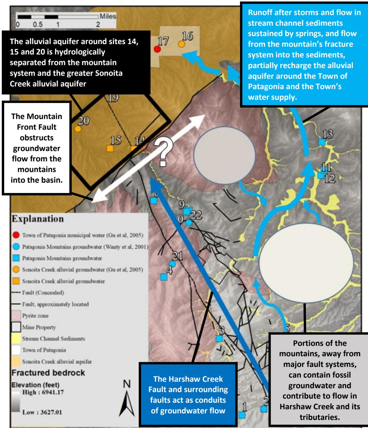
FIGURE 12: CONCEPTUAL MODEL OF GROUNDWATER FLOW IN THE NORTHERN PATAGONIA MOUNTAINS<sup>1</sup>
