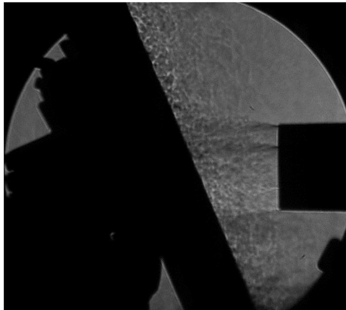
**Fig 4.3.1: Schlieren image of Nozzle 3 jet stream flow at  $U_e = 30\text{m/s}$  and impingement wall at  $\theta = 22.5^\circ$  seeded with CO<sub>2</sub>.**
