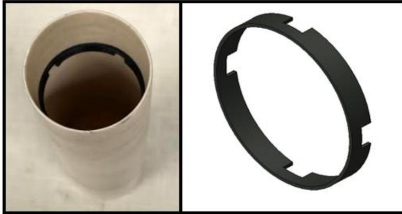
**Fig 2.3.3: Boundary layer trip ring installed in nozzle at 1” from the exit (left); 3D model of the trip ring (right).**
