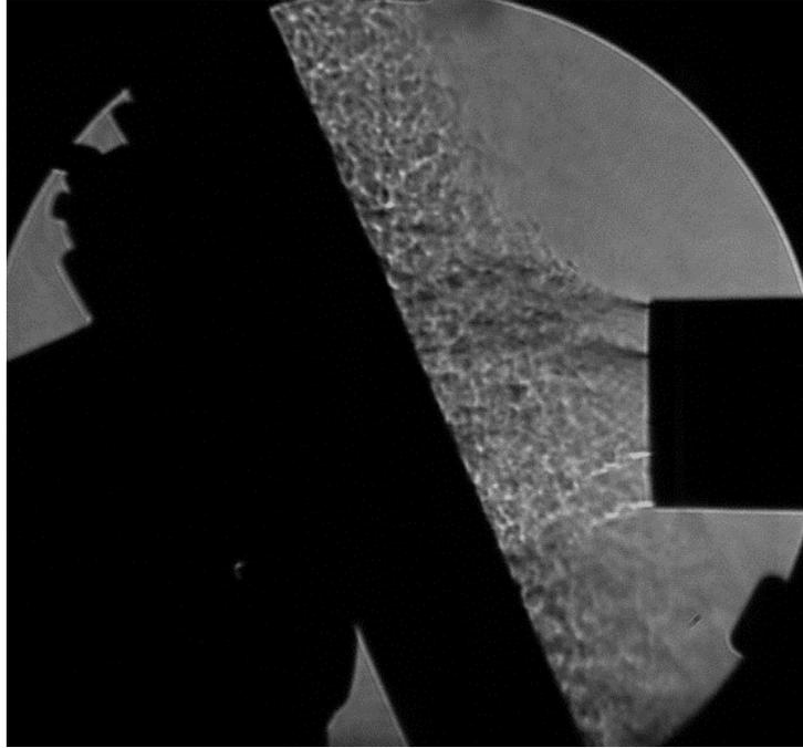
**Fig 4.3.7: Schlieren image of Nozzle 7 jet stream flow at  $U_e = 30\text{m/s}$  and impingement wall at  $\theta = 22.5^\circ$  seeded with  $\text{CO}_2$ .**
