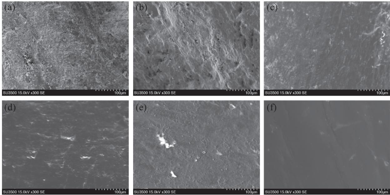
FIGURE 6: SEM images of different coal samples at a magnification factor of 300: (a) lignite; (b) gas coal; (c) fat coal; (d) coking coal; (e) meager-lean coal; (f) anthracite.
