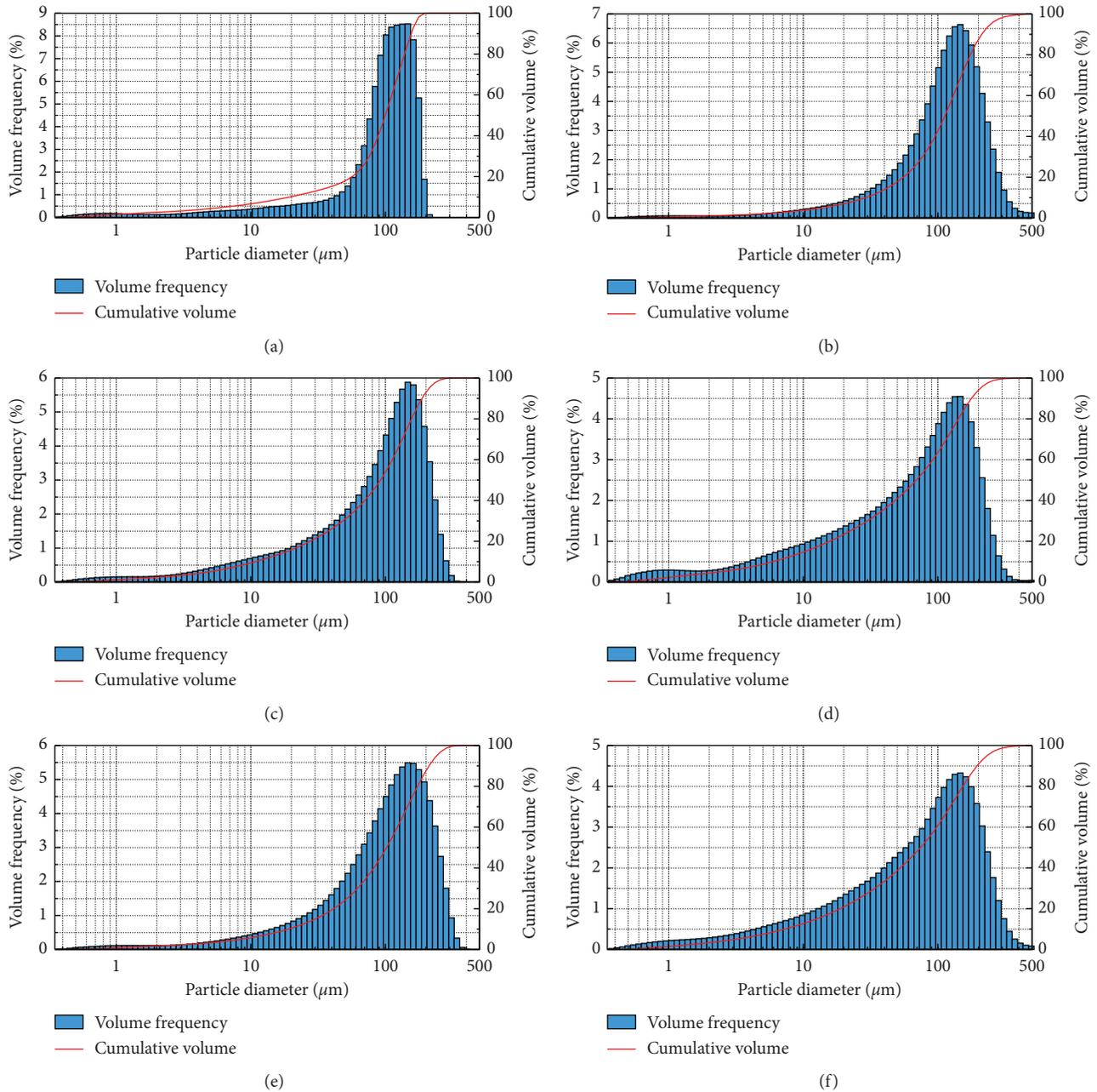
FIGURE 1: Particle size distribution of experimental coal samples: (a) lignite; (b) gas coal; (c) fat coal; (d) coking coal; (e) meager-lean coal; (f) anthracite.
