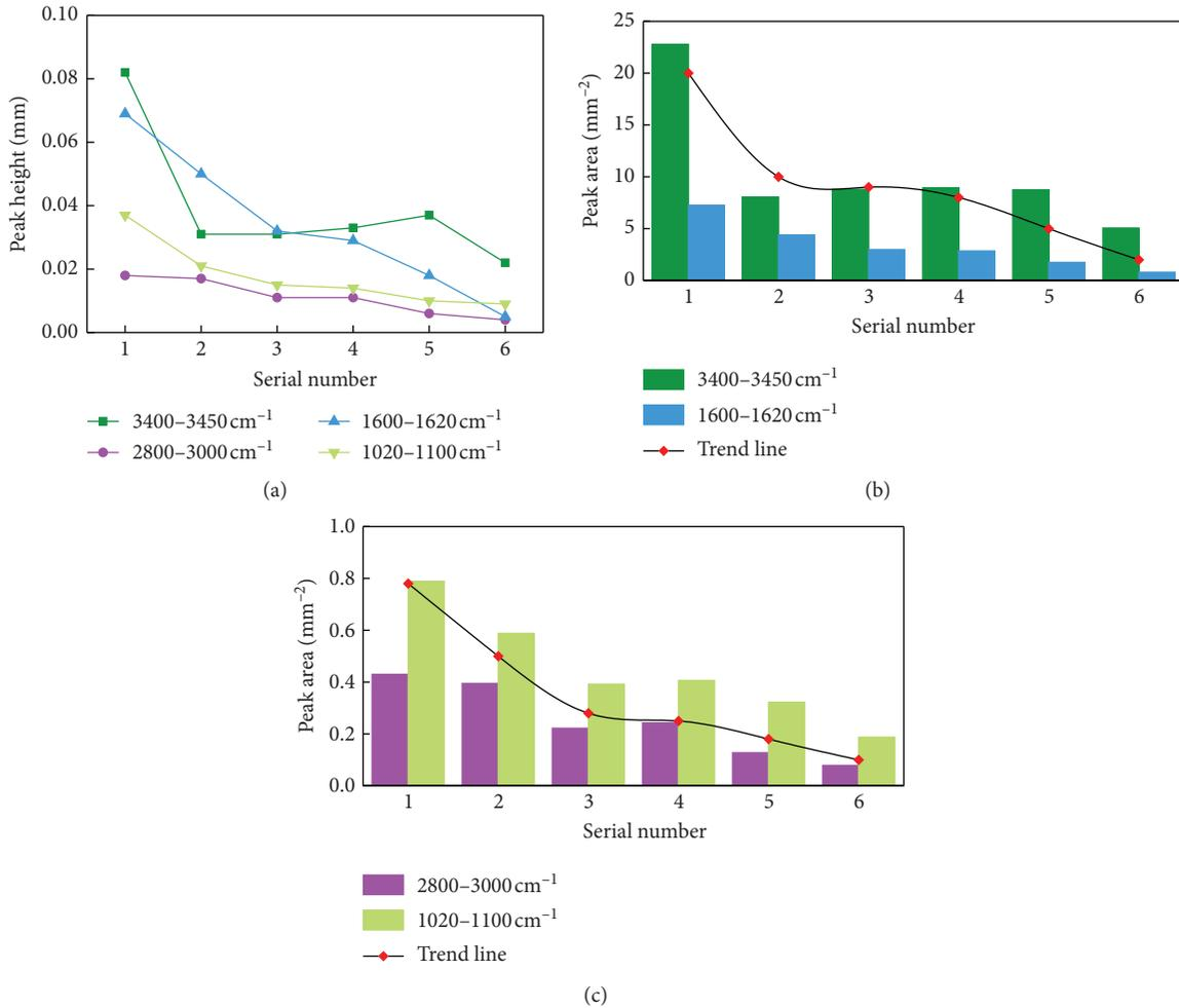
FIGURE 5: Heights and areas of the characteristic peaks of the oxygen-containing functional groups: (a) heights of the characteristic peaks; (b) areas at the characteristic peaks of  $3400\text{--}3450\text{ cm}^{-1}$  and  $1600\text{--}1620\text{ cm}^{-1}$ ; (c) areas at the characteristic peaks of  $2800\text{--}3000\text{ cm}^{-1}$  and  $1020\text{--}1100\text{ cm}^{-1}$ .
