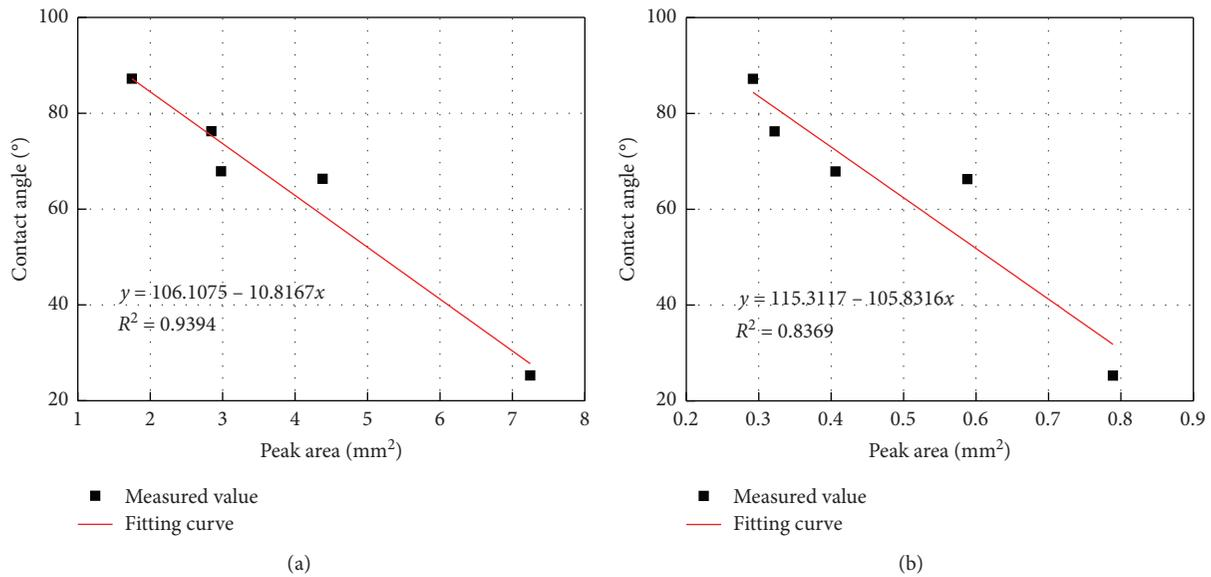
FIGURE 10: Relationship between the measured contact angle and the areas of the characteristic peaks: (a) 1600–1620 cm<sup>-1</sup>; (b) 1020–1110 cm<sup>-1</sup>.
