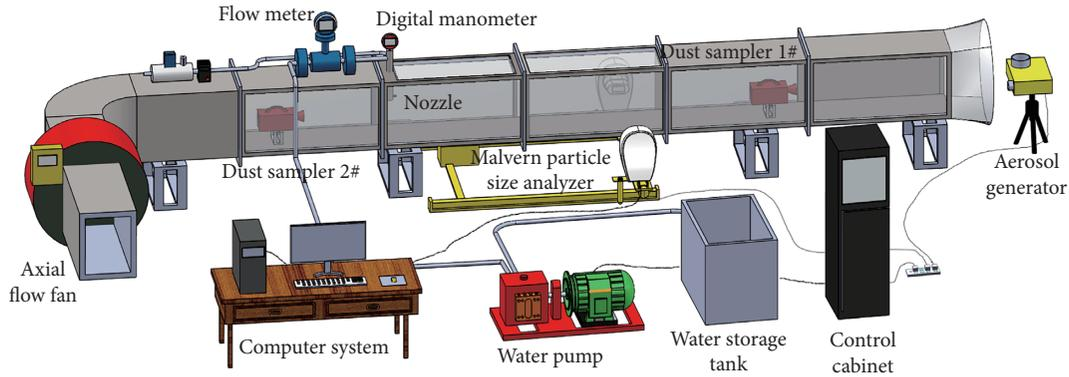
FIGURE 2: Dust-suppression experimental system via spraying.
