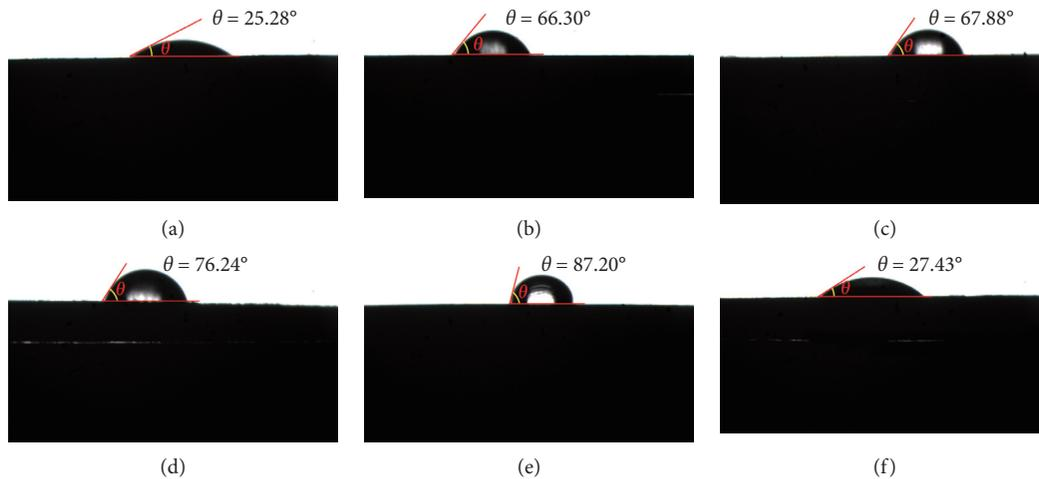
FIGURE 9: Measured contact angles for different coal samples: (a) lignite, (b) gas coal, (c) fat coal, (d) coking coal, (e) meager-lean coal, and (f) anthracite.
