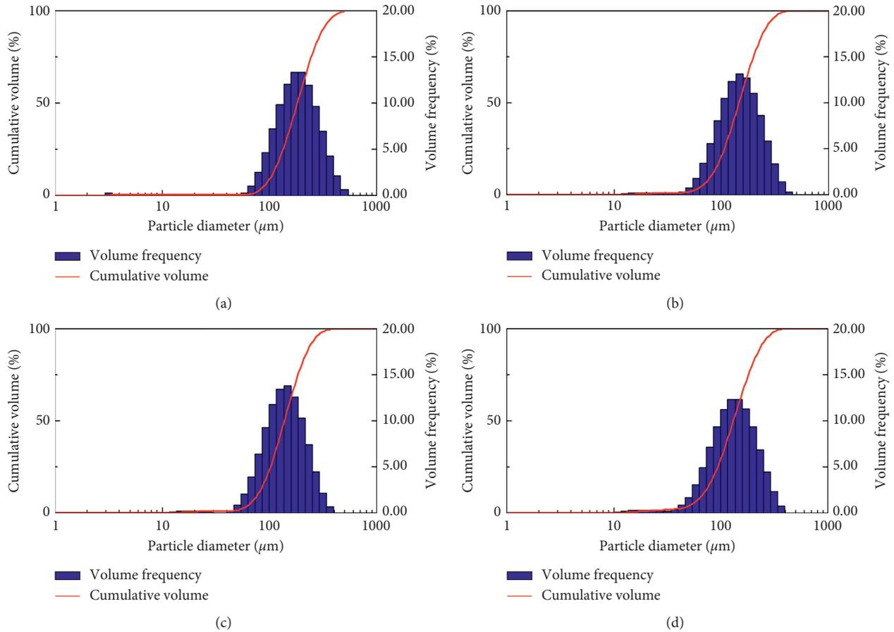
FIGURE 12: Distribution of droplet size under four different water-supply pressures: (a)  $p = 0.5$  MPa; (b)  $p = 1.0$  MPa; (c)  $p = 1.5$  MPa; (d)  $p = 2.0$  MPa.
