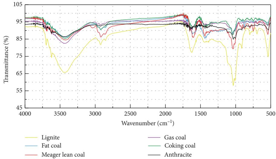
FIGURE 4: IR spectra of different coal dust samples.
