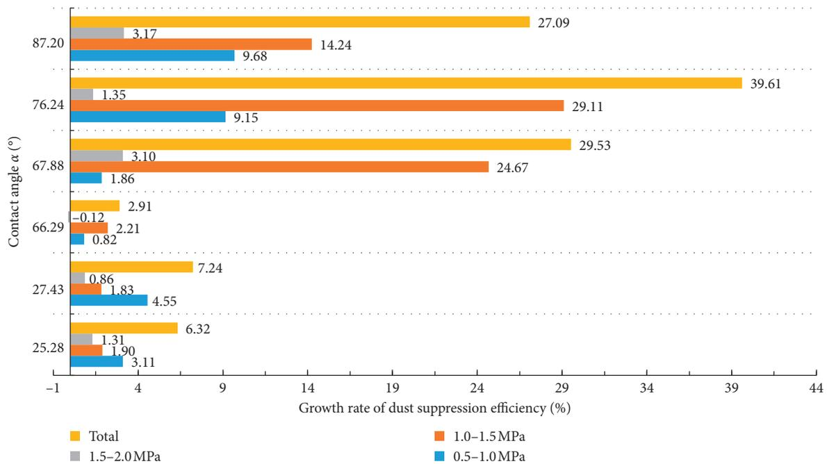
FIGURE 14: Relationship between dust-reduction efficiency via spraying and the contact angle of coal dust.
