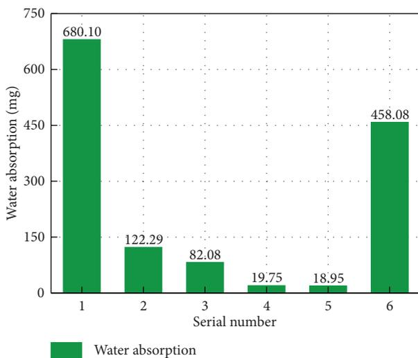
FIGURE 11: Water absorptions of different coal dust samples.
