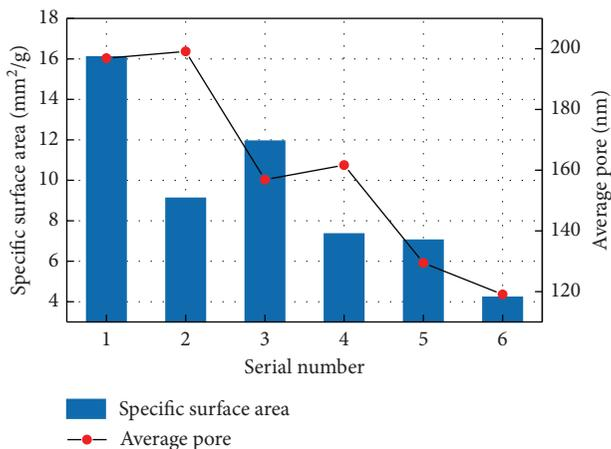
FIGURE 7: Specific surface area and mean pore diameter of coal samples with different metamorphic degrees.
