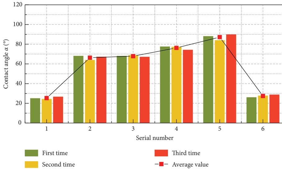
FIGURE 8: Measured contact angles of different coal dust samples.
