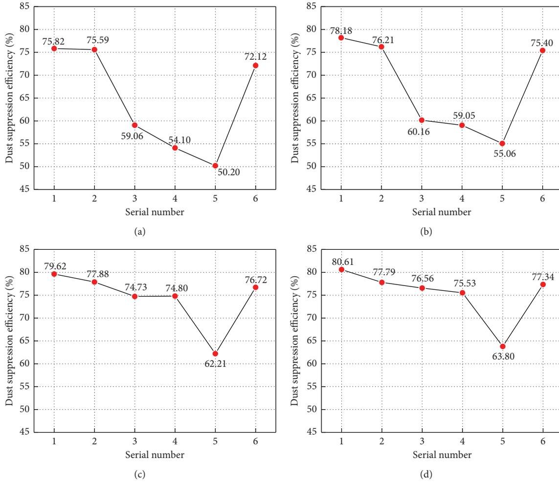
FIGURE 13: The dust-suppression efficiencies via spraying under different water-supply pressures: (a)  $p = 0.5$  MPa; (b)  $p = 1.0$  MPa; (c)  $p = 1.5$  MPa; (d)  $p = 2.0$  MPa.
