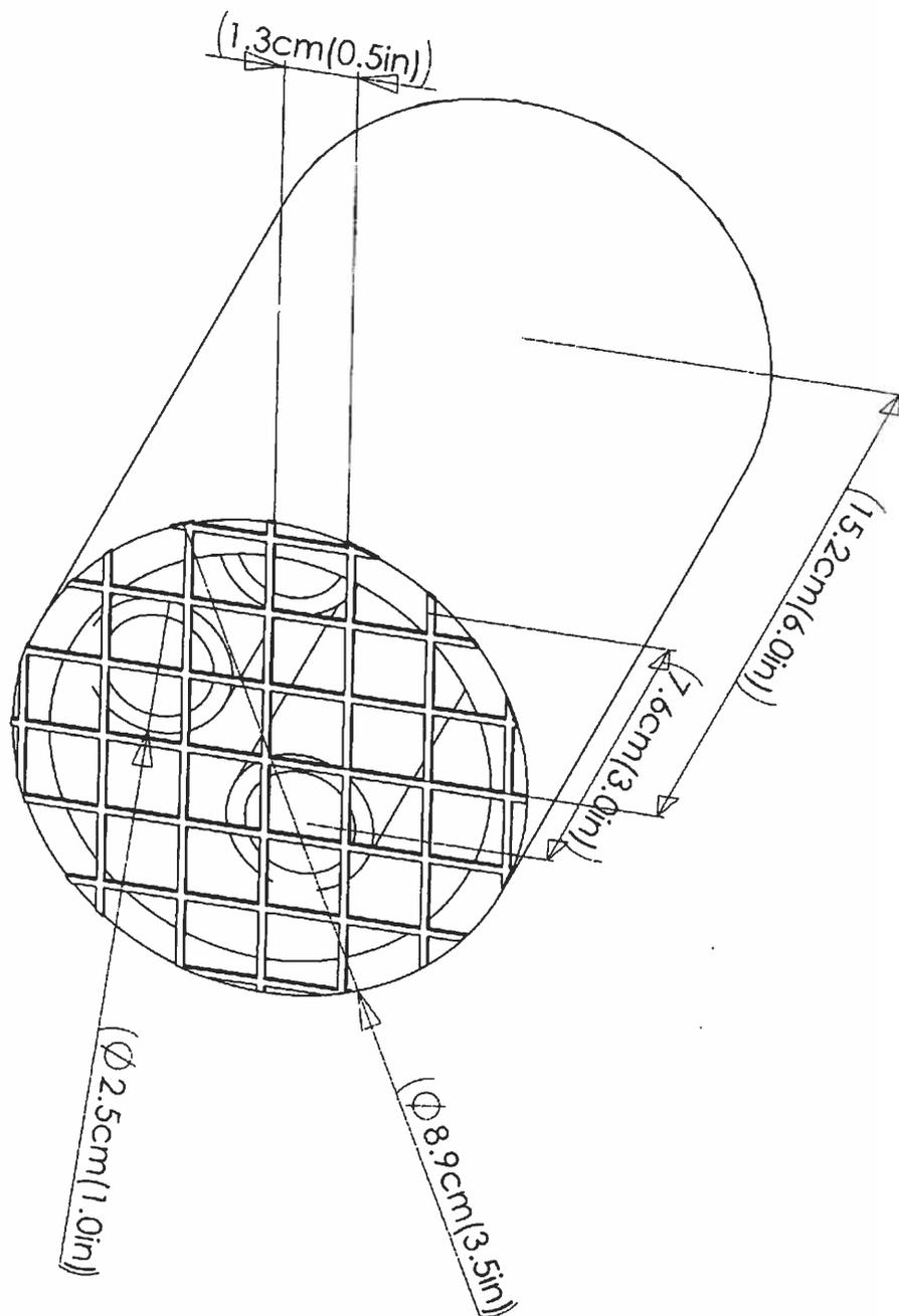
Fig. 1. Gully seeder design.
