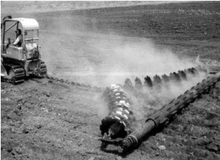
Fig. 2. Disk chain developed for single tractor pulling (Wiedemann and Cross 1985).
