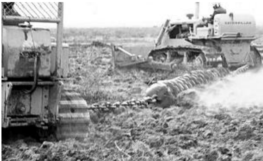
Fig. 1. Disk chain pulled between 2 crawler tractors for seedbed preparation on land littered with brush debris.
