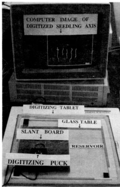
Fig. 1. Use of glass table with digitizing tablet for measuring axil length of germinants and seedlings.
