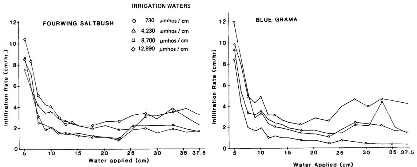
Fig. 3. Water infiltration rate of columns seeded to fourwing saltbush and blue grama over 37.5 cm of applied irrigation with waters ranging in EC from 730 to 12,890  $\mu\text{mhos/cm}$ .
