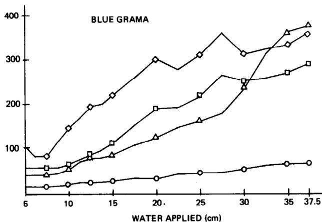
Fig. 4. Changes in electrical conductivity with additions of saline waters as determined by salinity sensors buried at 15 cm in columns in the greenhouse.
