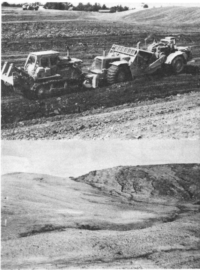
Fig. 2. Bentonite is mined with crawler tractors and scrapers, resulting in pits less than 5 ha in size (top). Old spoils, like this one mined in 1954, are steep, barren, and eroded (bottom).
