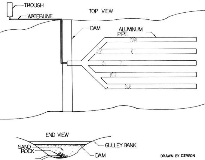
Fig. 1. A schematic design of a sand dam for harvesting overland flow; its storage and use by animals on arid lands.
