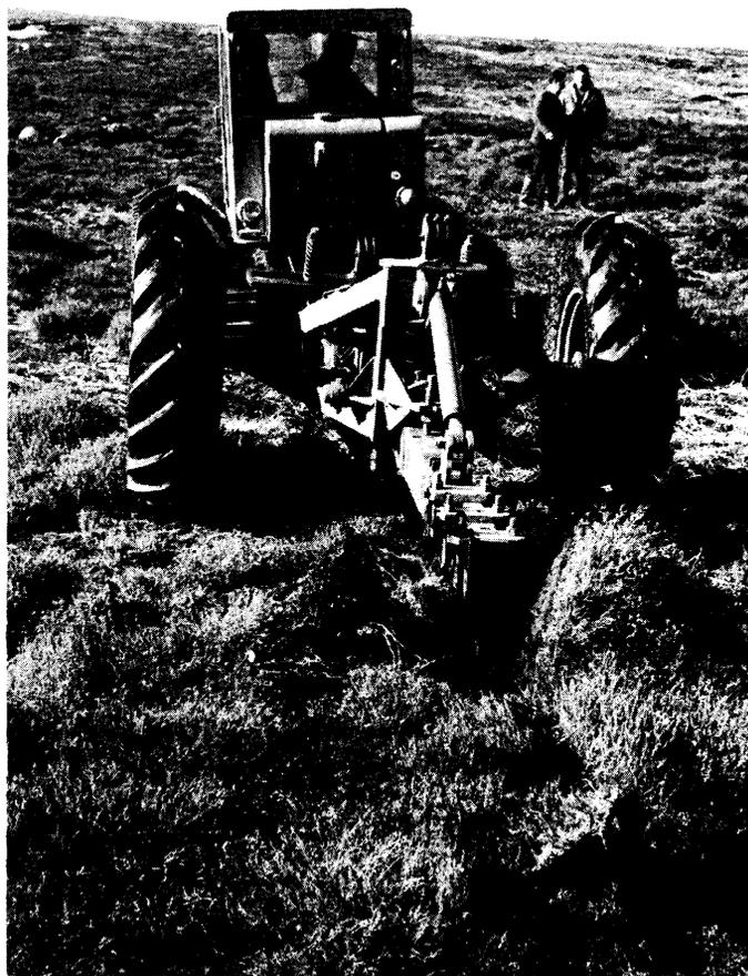
**Fig. 1.** Subsoiler in action on typical heather moor which can benefit from subsoil draining.
