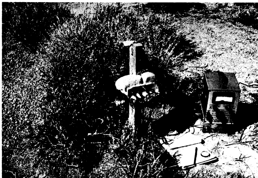
FIG. 1. Big sagebrush plant equipped for measuring sap flow velocities.
