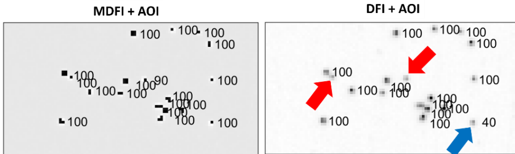
Figure 8. Fully automated AOI statistical results from 10 measurements. In the DFI results, two particles were missed completely (red arrow) and one was partially missed (blue arrow).
