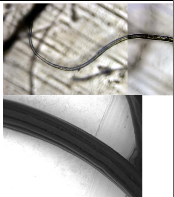
Fig. 2: Optical (top) and SEM (bottom) images of Fiber 2.
