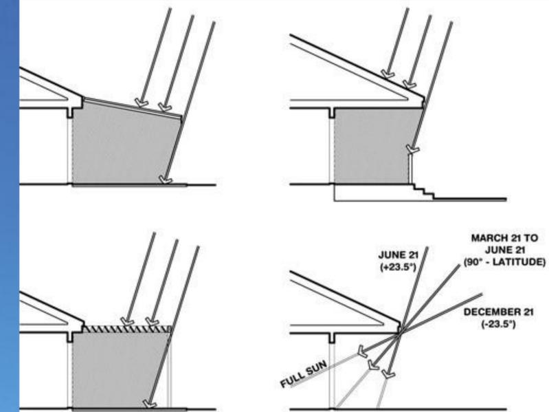
Figure 1. Overhang illustration to maximize shading in the summer and allow solar gain in the winter <sup>5</sup>
